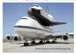
**Img. 6** A modified oeing 747 carrying the Space Shuttle Enterprise
