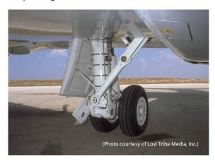
Img. 3 Trailing link landing gear
