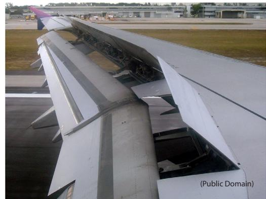
**Img. 1** Ground spoilers on an Airbus 320 aircraft
