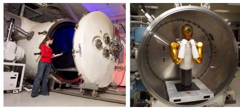
The White Sands flight acceptance workforce performs NASA Technical Standard "Flammability, Offgassing, and Compatibility Requirements and Test Procedures" and related customized testing designed to verify space flight materials and system performance with a focus on ensuring safety during manned space flights.
