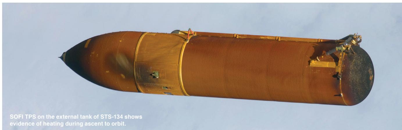
SOFI TPS on the external tank of STS-134 shows evidence of heating during ascent to orbit.
