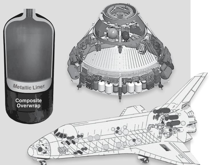
Illustrations of COPVs on an orbiter and the Orion crew module.
