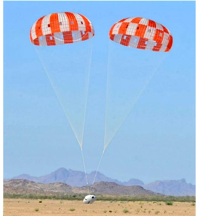
Drop test using only two of three CPAS main parachutes.
