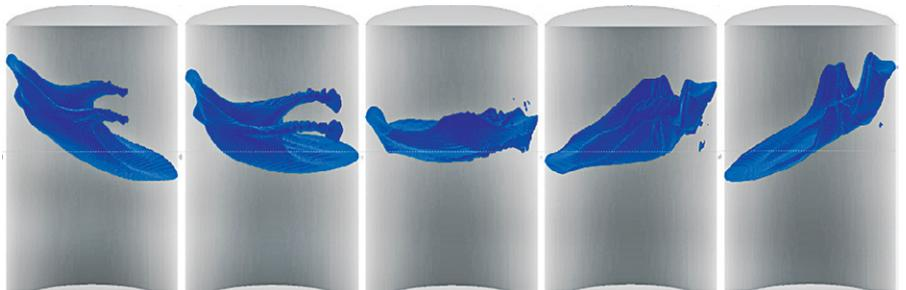
Simulation of slosh in a cylindrical tank.
