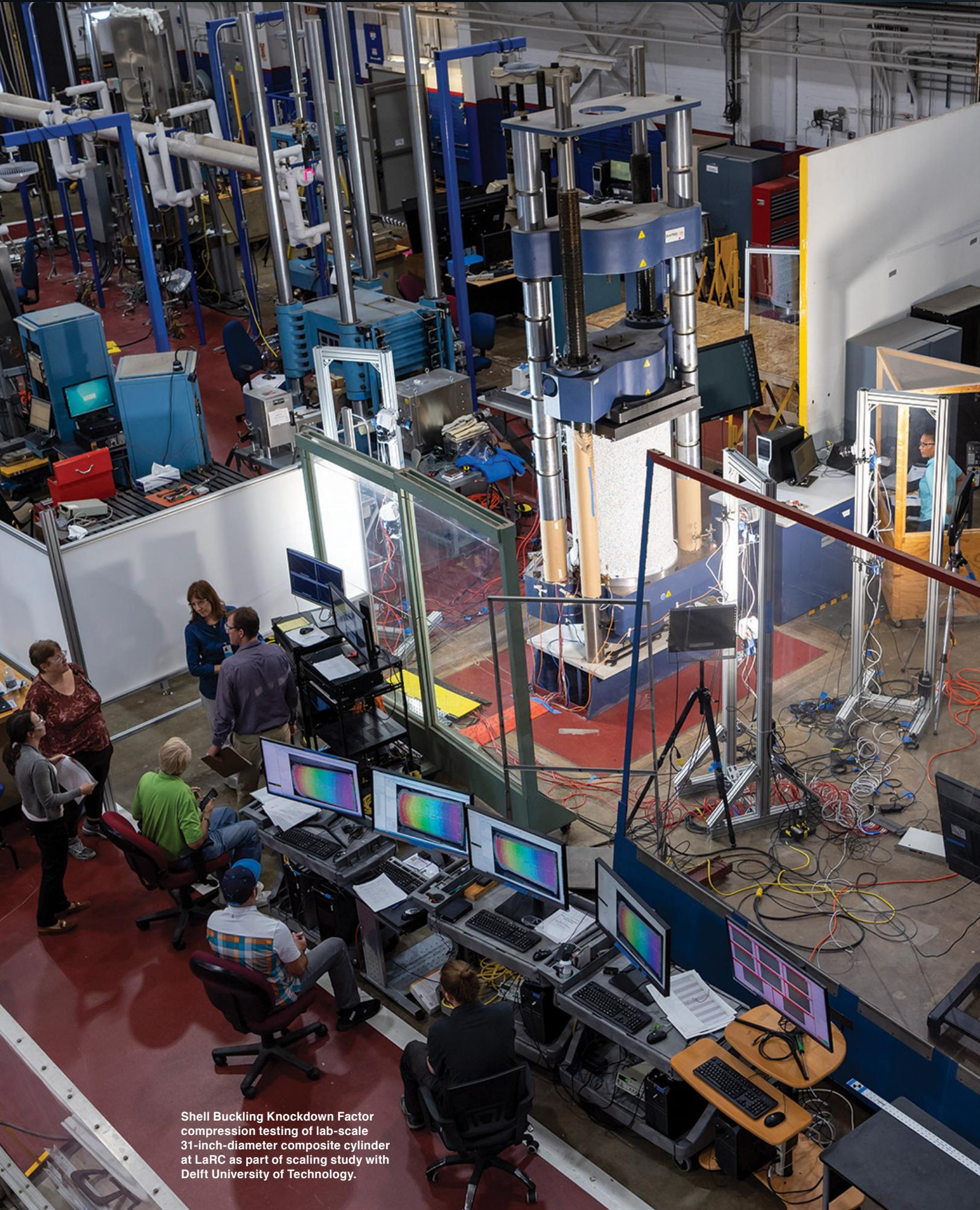
Shell Buckling Knockdown Factor compression testing of lab-scale 31-inch-diameter composite cylinder at LaRC as part of scaling study with Delft University of Technology.
