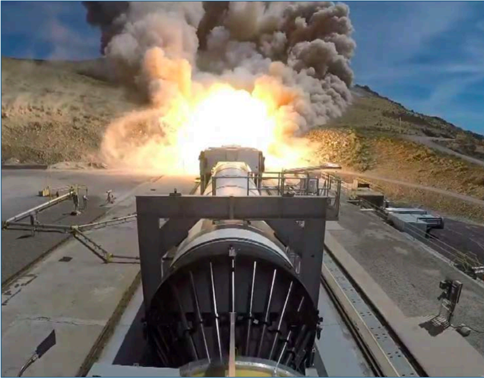
NASA and Northrop Grumman successfully complete the Flight Support Booster-1 (FSB-1) test in Promontory, UT, on Sept. 2. The full-scale booster firing was conducted with new materials and processes that may be used for NASA's Space Launch System (SLS) rocket boosters.
