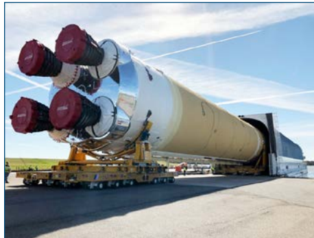
The Core Stage being loaded onto Pegasus at the Michoud Assembly Facility
