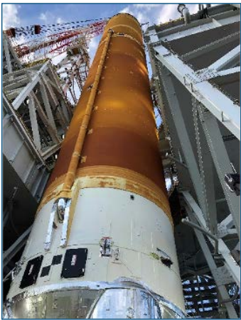
SLS Core Stage removal from SSC B2 Test Stand
