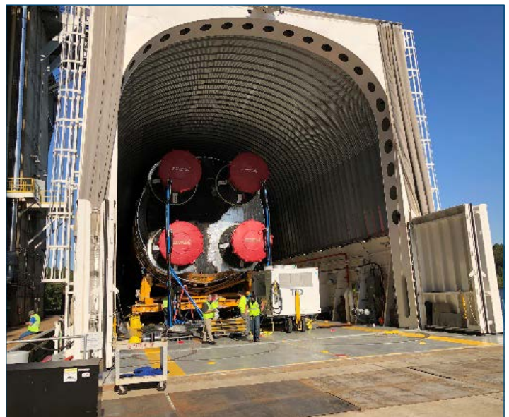
SLS Core Stage loading into Pegasus at SSC
