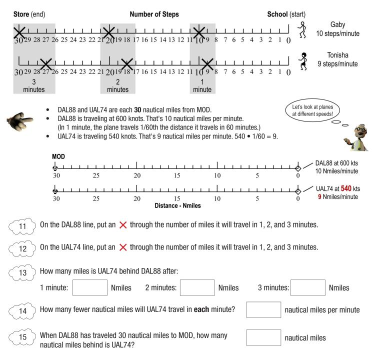
• At 600 knots, a 60-knot speed drop causes a 1 nautical mile distance drop every *minute*.
