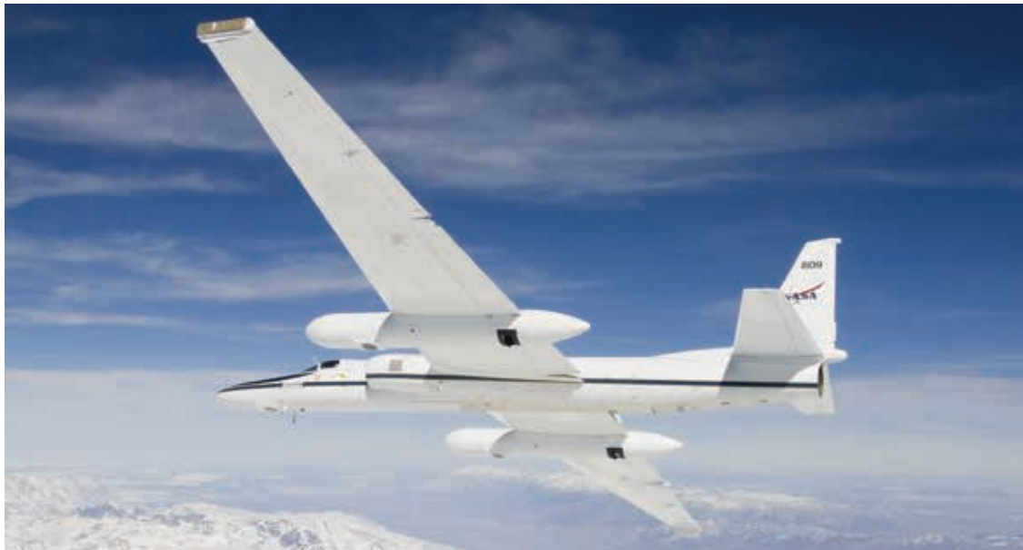
NASA operates two Airborne Science ER-2 aircraft for a wide variety of environmental science, atmospheric sampling, and satellite data verification missions. NASA/Carla Thomas
