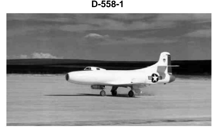
The D-558-I "Skystreaks" were among the early transonic research airplanes like the X-1, X-4, X-5, and XF-92A. Three of the single-seat, straight-wing aircraft flew in a joint program involving the National Advisory Committee for Aeronautics (NACA), the Navy-Marine Corps, and the Douglas Aircraft Co. from 1947 to 1953. In the process, the Skystreaks set several world speed records.
