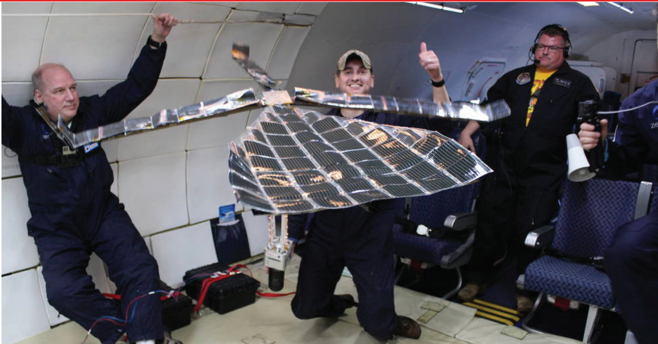
Image: Successful deployment of a LISA-T thin film solar array on a parabolic flight provided by Zero Gravity Corporation in November 2019. Credits: NeXolve Holding, LLC
