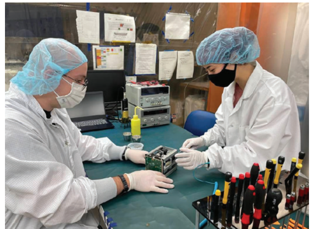
Image details: Graduate students build the test assembly of the CubeSat Laser Infrared Crosslink, or CLICK, B/C engineering development unit in a clean room at the Massachusetts Institute of Technology in Cambridge. Credit: Massachusetts Institute of Technology
