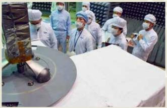
The HTV5 CALorimetric Electron Telescope (CALET) Flight Crew Interface Test (FCIT). CALET will search for signatures of dark matter and provide the highest energy direct measurements of the cosmic ray electron spectrum.
