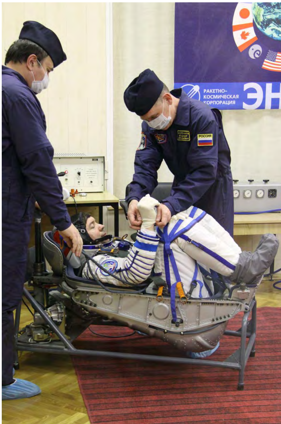
Astronaut Michael Barratt, NASA Expedition 19 flight engineer, undergoes a pressure and leak check on his Russian launch and entry suit at the Baikonur Cosmodrome in Kazakhstan (March 12, 2009).
