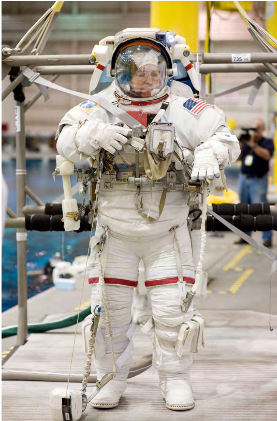
Attired in a training version of his Extravehicular Mobility Unit spacesuit, astronaut Michael Barratt, Expedition 19/20 flight engineer, awaits the start of a spacewalk training session in the waters of the Neutral Buoyancy Laboratory near NASA's Johnson Space Center.
