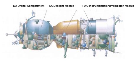
The Soyuz spacecraft is launched to the space station from the Baikonur Cosmodrome in Kazakhstan aboard a Soyuz rocket. It consists of an Orbital Module, a Descent Module and an Instrumentation/Propulsion Module.
