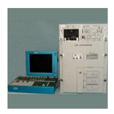
The only maintenance to be performed by Space Station crewmembers on the ultrasound system is vacuuming an inlet air debris screen as necessary.
