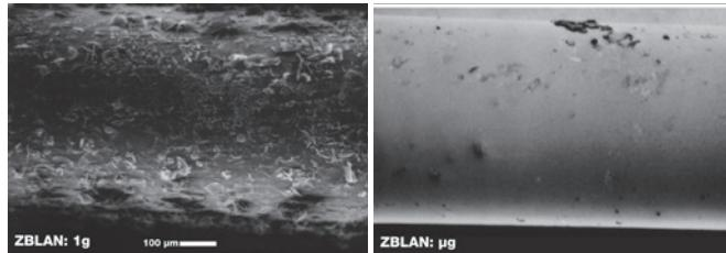
This scanning electron microscope image shows the surface defects caused by crystallization of ZBLAN fibers pulled on Earth (left) versus in microgravity (right). Flight Opportunities is investing in flight testing of space-based manufacturing methods for ZBLAN fibers to take advantage of the superior end result that may be achieved in space. Credit: NASA's Marshall Space Flight Center
