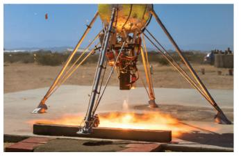
Masten's Xodiac lifts off from a launchpad in Mojave, California, for testing of Flight Opportunities-supported technologies. PlanetVac can be seen attached to the lander leg in the foreground. Credit: Masten Space Systems
