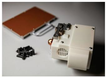
A preflight view of the RRP suite, which arrived at the station aboard NG-16. The suite includes print heads, plates, and lunar regolith simulant feedstock. Credit: Redwire Space
