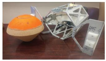
The KREPE capsule (left) can carry small samples, instruments, and other cargo from low-Earth orbit back to Earth. Its metal enclosure opens to release it at the appropriate altitude. Credit: University of Kentucky
