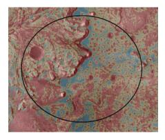
The Mars 2020 Perseverance rover relied on data depicted in this hazard map to help guide it to a safe landing. Safer landing areas are colored blue and green. To select the best location to touch down while avoiding damage to the rover. the spacecraft's TRN-based system took images of the terrain below during Perseverance's descent. Credit: NASA
