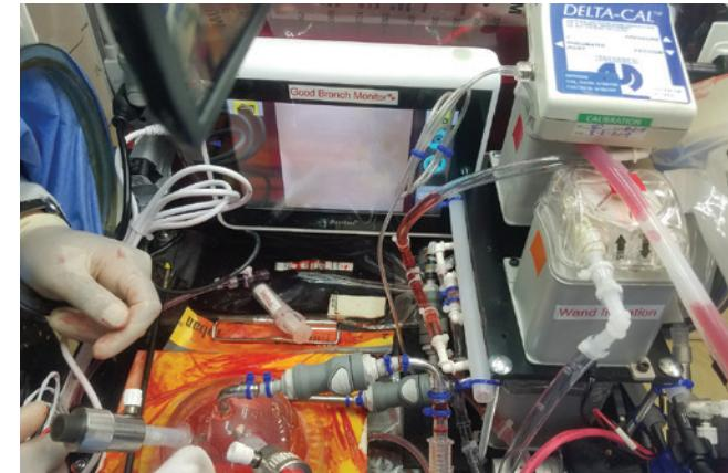
Automation of a surgical system designed for wound care was tested in space on Virgin Galactic's SpaceShipTwo. On parabolic flights (shown here), the simulated surgical procedure was performed by researchers. Credit: University of Louisville
