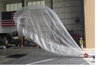
Raven Aerostar's Zero Pressure Balloon System is inflated for a launch to carry the NephEx pavload on June 11, 2021, Credit: Raven Aerostar
