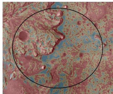
The Mars 2020 Perseverance rover relied on data depicted in this hazard map to help guide it to a safe landing. Safer landing areas are colored blue and green. To select the best location to touch down while avoiding damage to the rover, the spacecraft's TRN-based system took images of the terrain below during Perseverance's descent. Credit: NASA
