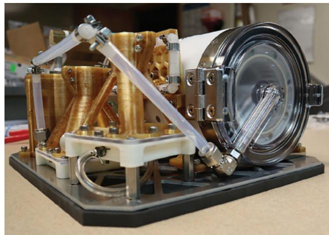
The microgravity LilyPond was one of several space technologies tested on New Shepard. The growth chamber uses capillary action to provide a stable water surface on which plants can grow. Credit: Space Lab Technologies
