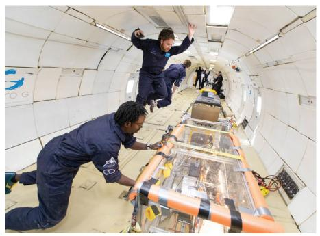
Researchers from University of Colorado Boulder leveraged parabolic flights to test a direct writing technique that could be used for in-situ lunar manufacturing of life support systems. Note: Flight participants were required to provide proof of vaccination or negative COVID-19 test results prior to flight. Credit: Zero Gravity Corporation/ Steve Boxall
