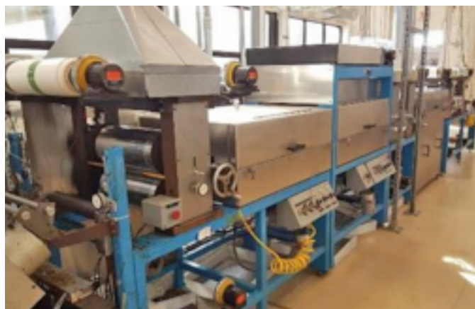
NASA researchers print the experimental adhesive using a special prepregger tape machine.
