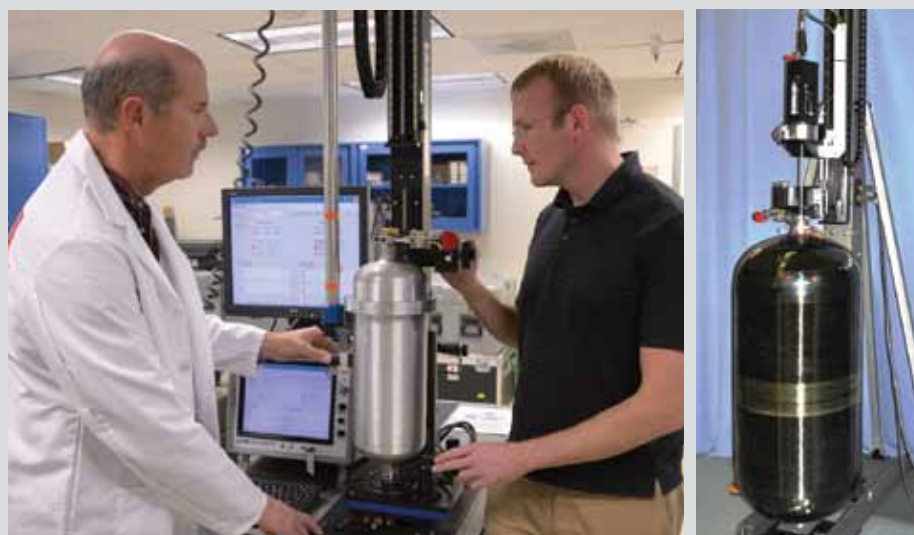
(Left photo) WSTF personnel, Paul Spencer, left, and Charles Nichols, right, configure a desktop system to do EC scanning of a liner defect standard. (Right photo) A 48-inch Orion service module CPV simulator in the tall delivery stage.
