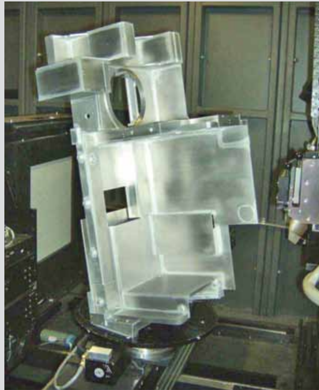
CrIS frame during x-ray computed tomography inspection.
