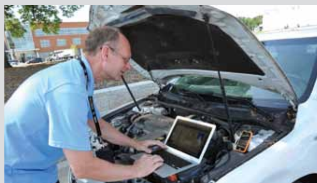
Michael Bay examines engine response to accelerator inputs using Toyota's onboard diagnostic port.
