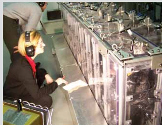
Dr. Lorie Grimes-Ledesma examines composite pressure vessels undergoing life testing at WSTF.
