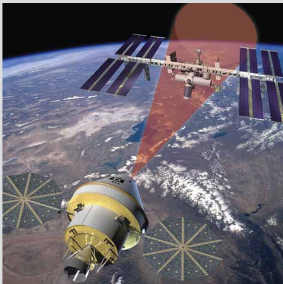
A notional representation of the VNS flash LIDAR illuminating the ISS to determine range and bearing relative navigation information.
