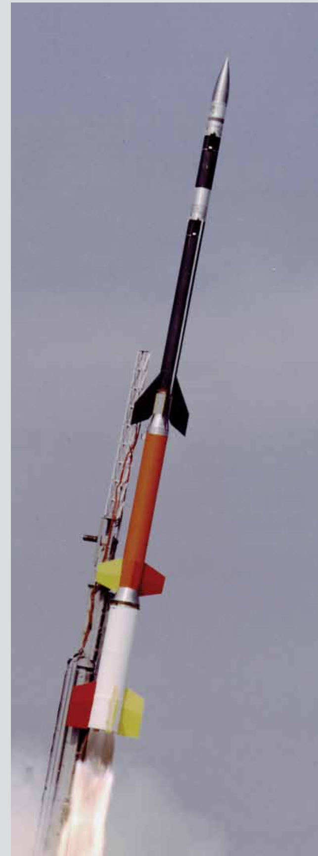
The Black Brant sounding rocket motor (black upper stage), operational since the 1960s, is the workhorse of NASA's Sounding Rocket Program.
