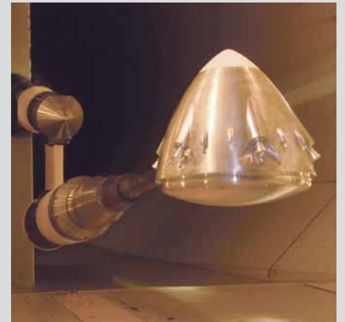
An MLAS objective system configuration undergoing wind tunnel test at LaRC's Transonic Dynamics Tunnel.
