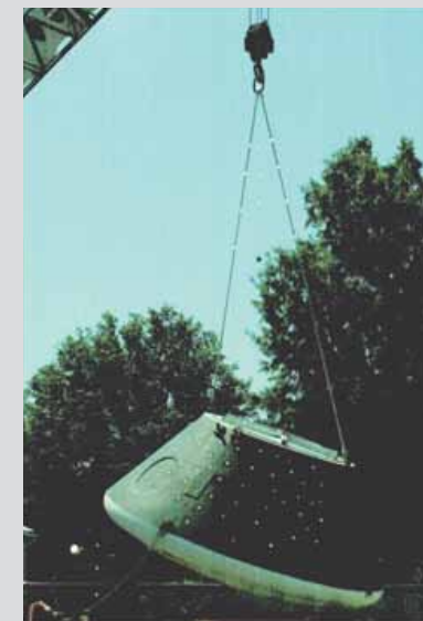
Figure 1. CM in CG test configuration with plumb line(s).
