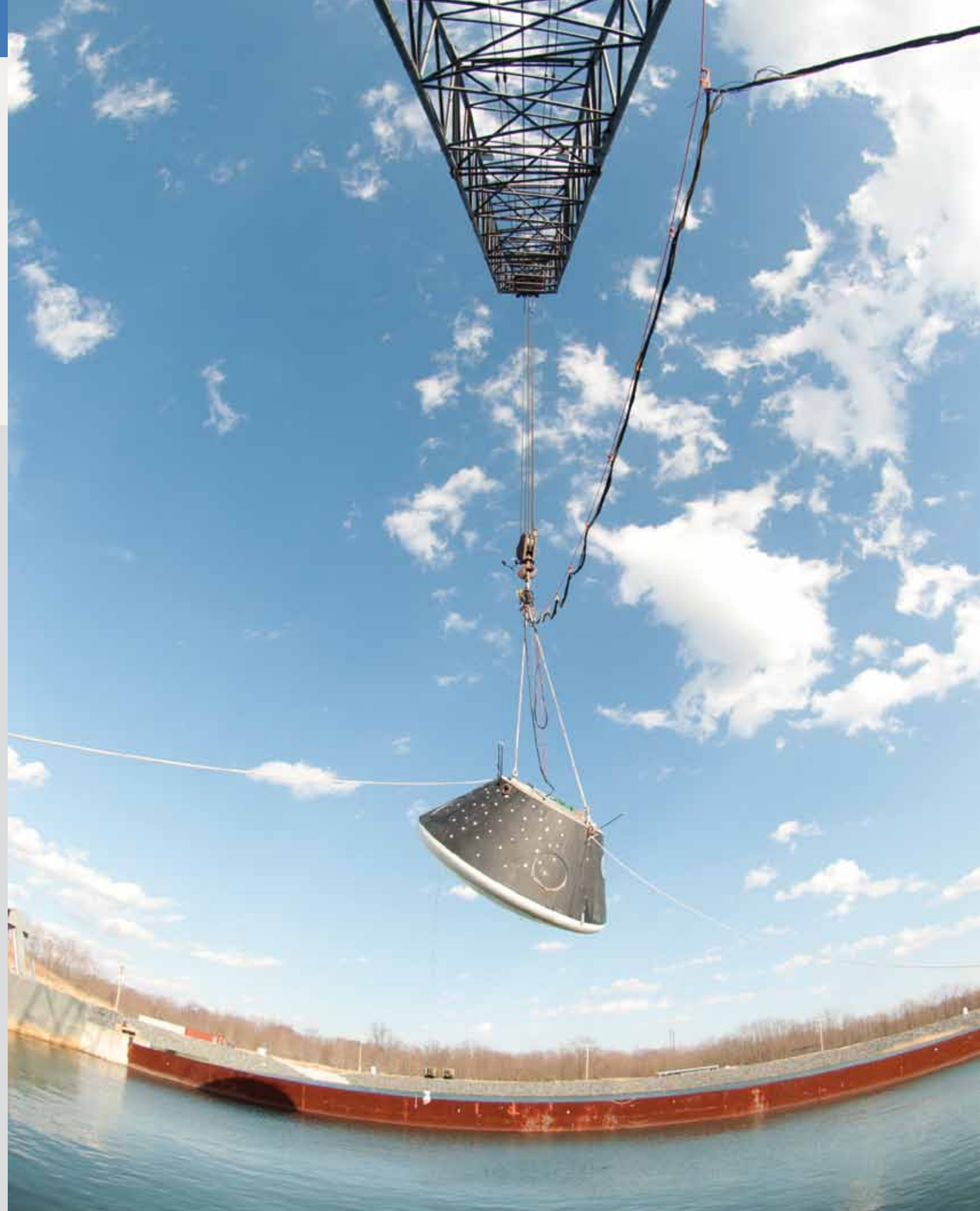
The NESC’s boilerplate Orion crew module is hoisted to drop height
