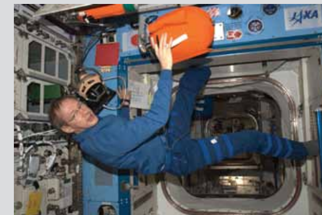
An ISS Expedition 20 flight engineer conducts an inspection on portable fire extinguisher and portable breathing apparatus equipment.
