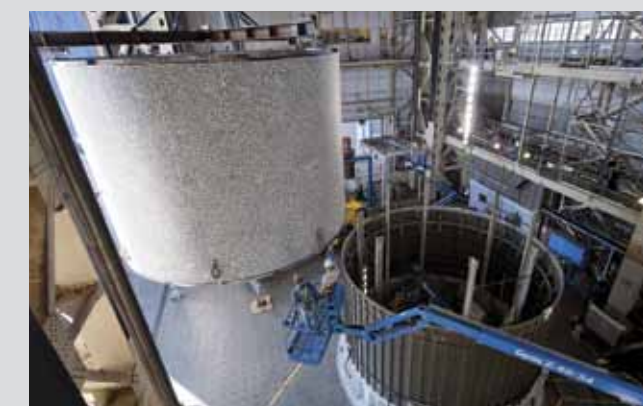
A section of a space shuttle external tank covered in photogrammetry targets shown mounted in the shell buckling test fixture.
