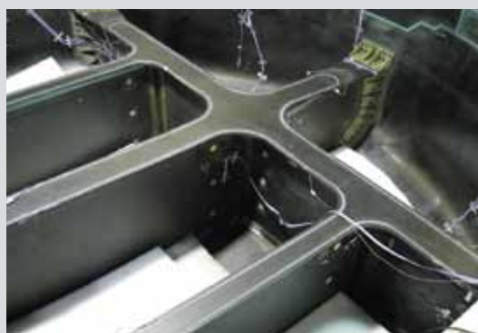
Fiber optic strain measurement system
