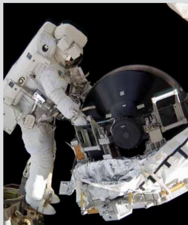
The CMG-3 was replaced during STS-118 mission to the ISS.
