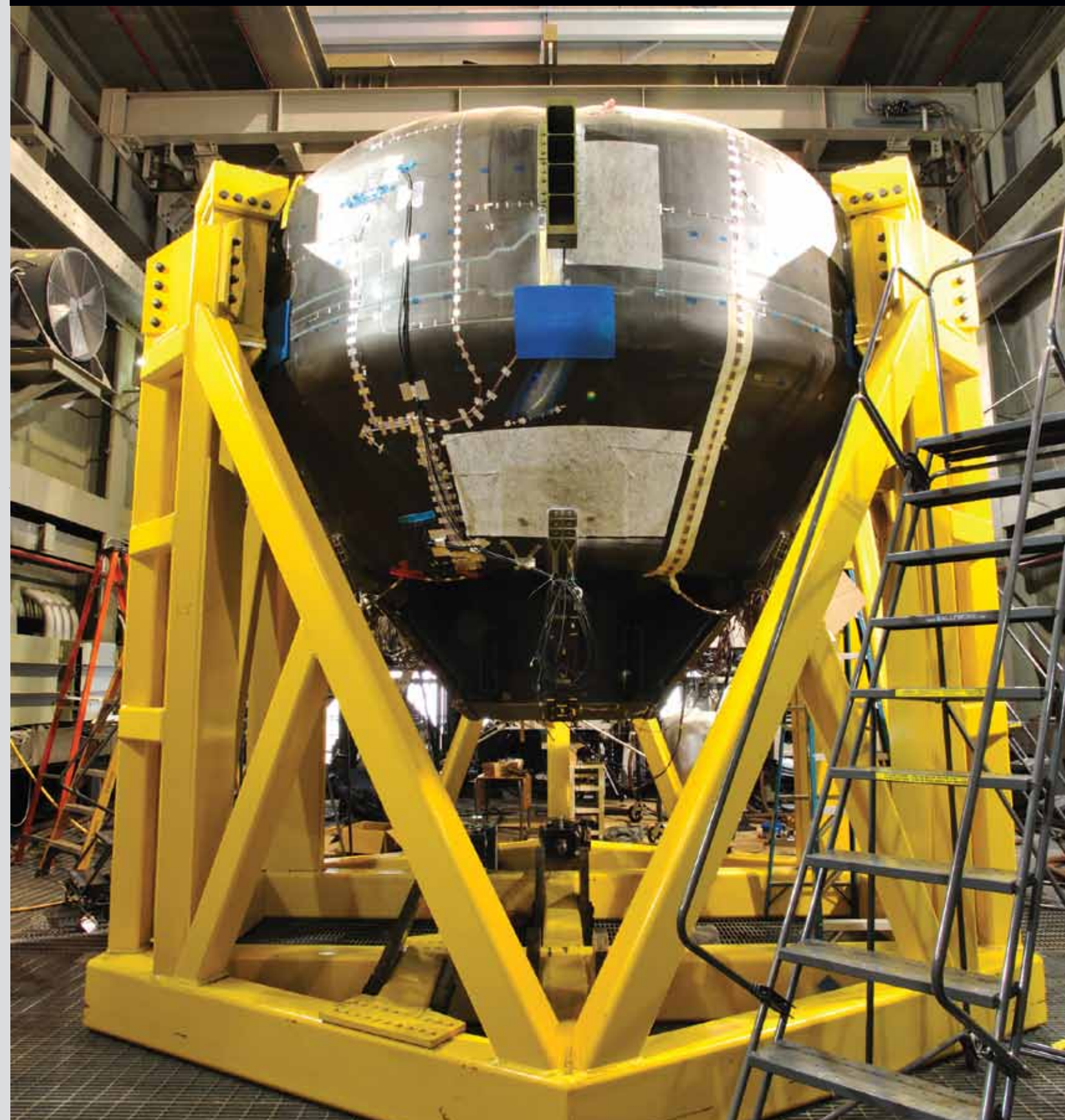
The composite crew module underwent destructive testing in LaRC's Combined Loads Testing Facility
