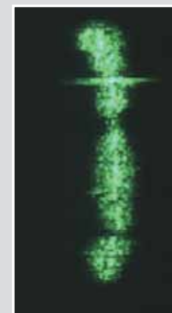
Penetrant indication for tightly closed (0.088-inch) fatigue crack in a propellant tank.
