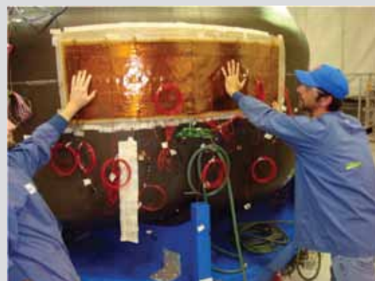
Out of autoclave, Kapton heater localize material curing and repair system
