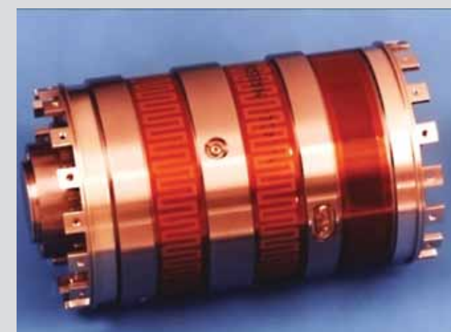
An HST gyro showing the heaters (2 bands on left) and secondary temperature sensor (on right).
