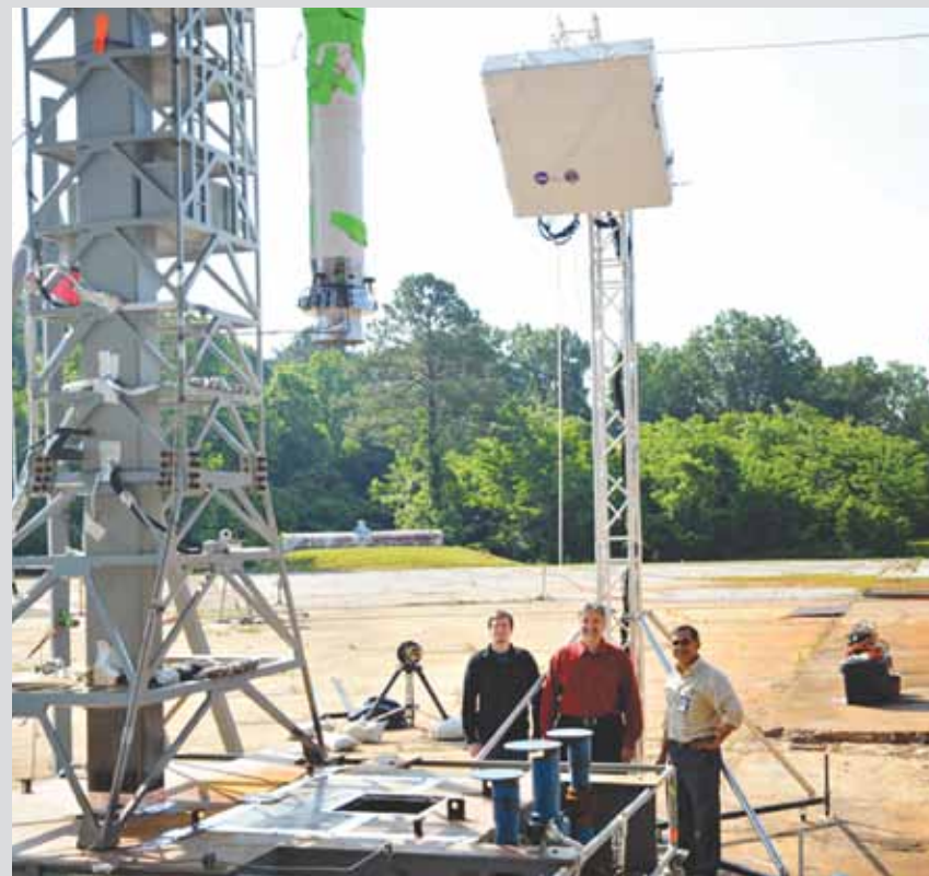
(From left) Robert Mosher, Roberto Garcia, and Jayanta Panda in front of the acoustic phased-array sensor tower, viewing the Ares I scale launch vehicle and launch pad model.
