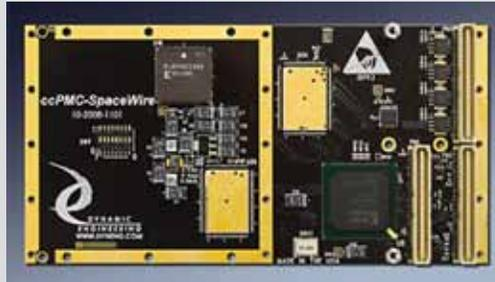
Spacewire printed circuit board.
