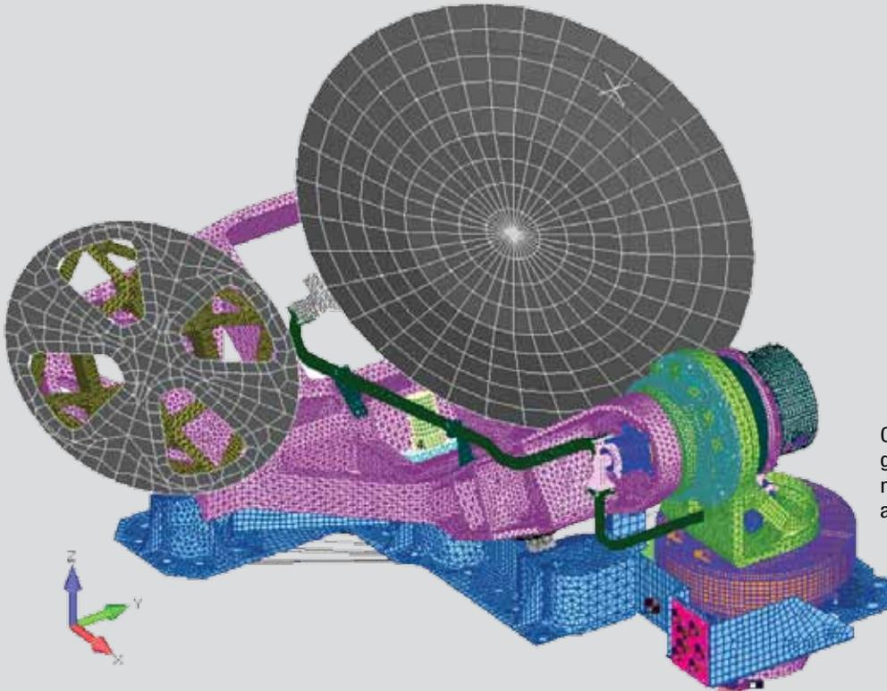
CoNNeCT antenna gimbal finite element model used in the analysis.
