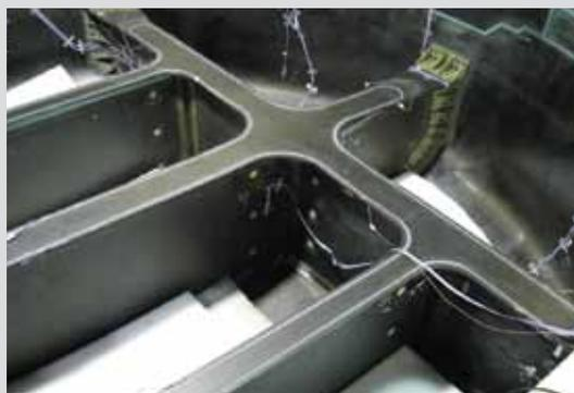
Fiber optic strain measurement system
