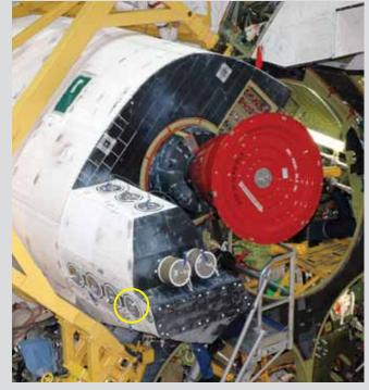
Orbital maneuvering system showing the L1L thruster (circled).
