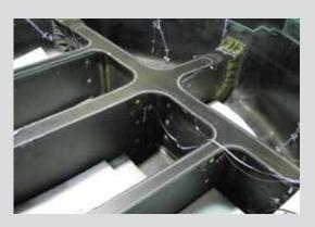
Fiber optic strain measurement system
