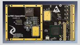
Spacewire printed circuit board.
