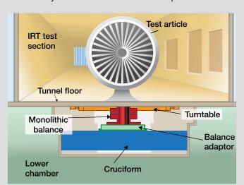
NESC recommended concept for GRC IRT FMS includes a new monolithic balance and balance adaptor and modifications to the existing turntable and cruciform.
