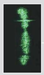
Penetrant indication for tightly closed (0.088-inch) fatigue crack in a propellant tank.
