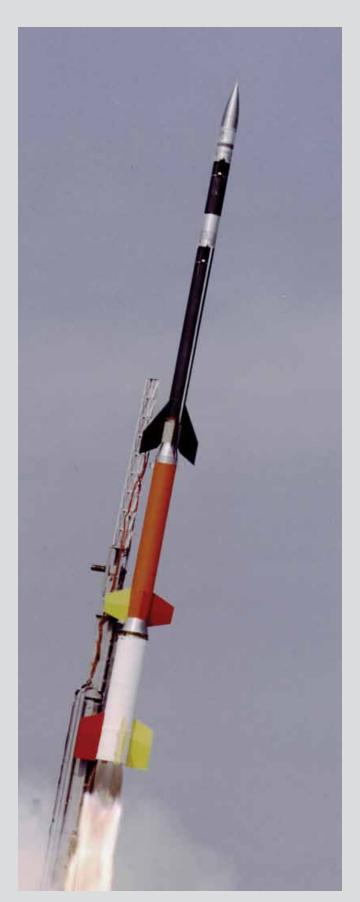
The Black Brant sounding rocket motor (black upper stage), operational since the 1960s, is the workhorse of NASA's Sounding Rocket Program.
