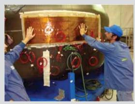
Out of autoclave, Kapton heater localize material curing and repair system
