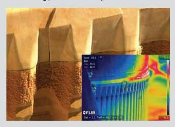
Visible-light and infrared (inset) photographs of ET foam crack.
