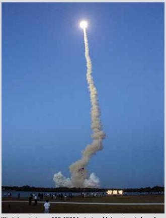
Wind shear between 500-1000 feet, viewable by exhaust plume from STS-119 launch on March 15, 2009.
