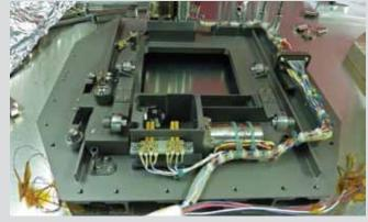
NIRSpec microshutter subsystem life test unit.
