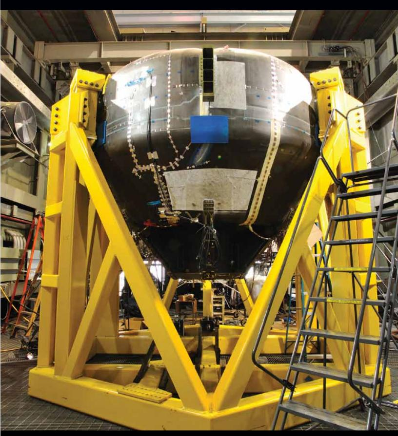
The composite crew module underwent destructive testing in LaRC's Combined Loads Testing Facility
