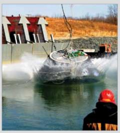
Both phases of water impact testing were completed at the U.S. Army's Aberdeen Test Center, Maryland.
