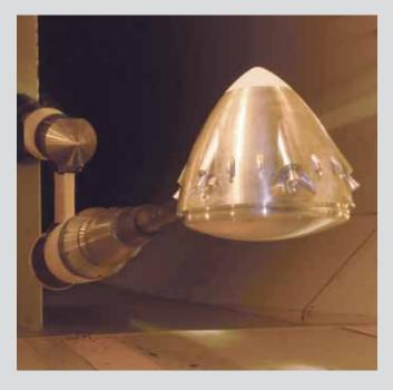
An MLAS objective system configuration undergoing wind tunnel test at LaRC's Transonic Dynamics Tunnel.
