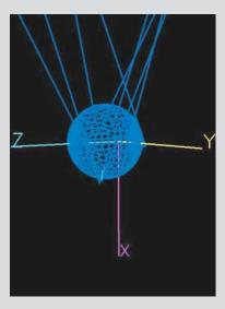
Figure 3. Intersecting plumb lines at CG. Inclusive sphere radius 0.667 inches. Center offset from origin 0.367 inches.
