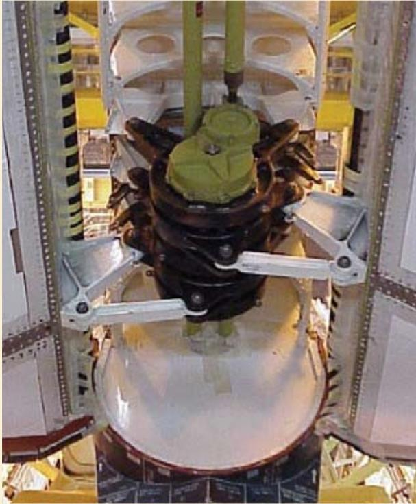
*Rudder/Speed Brake Actuator installed in an Orbiter tail section*
