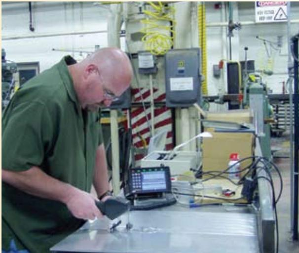
*Chris McGougan, Marshall Space Flight Center, performs a weld peaking and mismatch measurement of a simulated International Space Station Aluminum Variable Polarity Plasma Arc weld*
