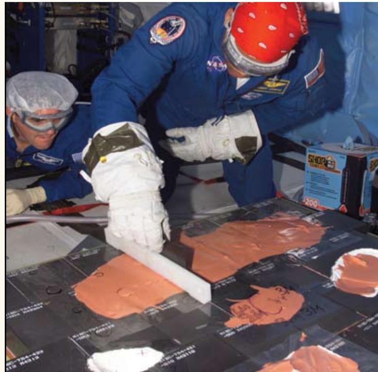
*Onboard a KC-135 aircraft, astronaut Robert L. Curbeam rehearses extravehicular activity tasks for repairing damaged Shuttle tiles*
