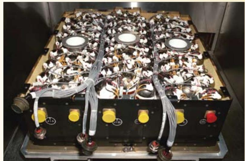
*Nickel hydrogen battery ground test unit undergoing long term capacity testing at the Marshall Space Flight Center*
