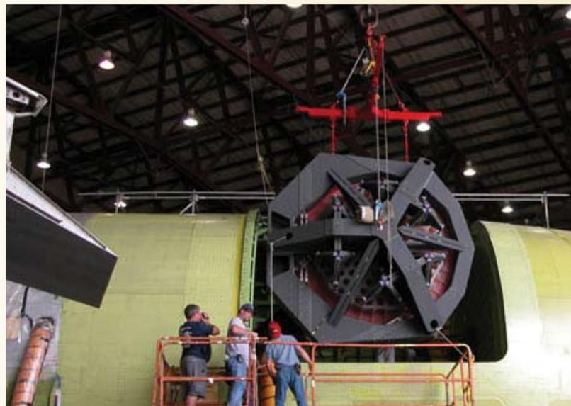
Workers lower the infrared telescope into the cavity of the NASA Boeing 747SP (photo courtesy of L3)
