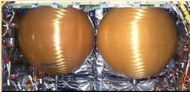
*Gaseous nitrogen Composite Overwrapped Pressure Vessels installed in the Orbiter environmental control and life support system*
