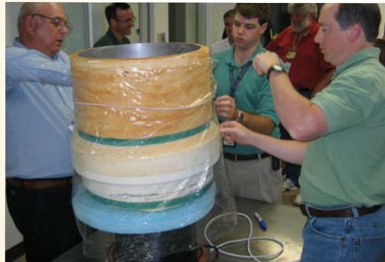
*Kennedy Space Center Engineers Charlie Stevenson, left, Wesley Johnson, center, and James Fesmire, right, install shrink wrap on a liquid oxygen bellows test article prior to cryogenic testing*
