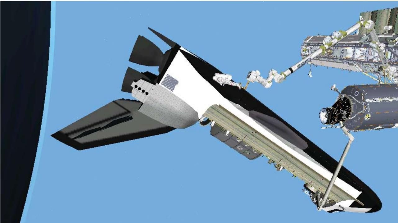
*Illustration of Orbiter Thermal Protection System repair extravehicular activity; the Orbiter maintains position with its arm while the astronaut is on the end of the International Space Station arm*
