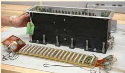
*Engine Cut-Off Point Sensor Electronics Box stimulates ECO Sensors and conditions signals received from them for processing by the Orbiter and ground computers*
