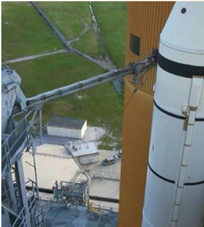
*Hydrogen vent arm in the launch configuration*
