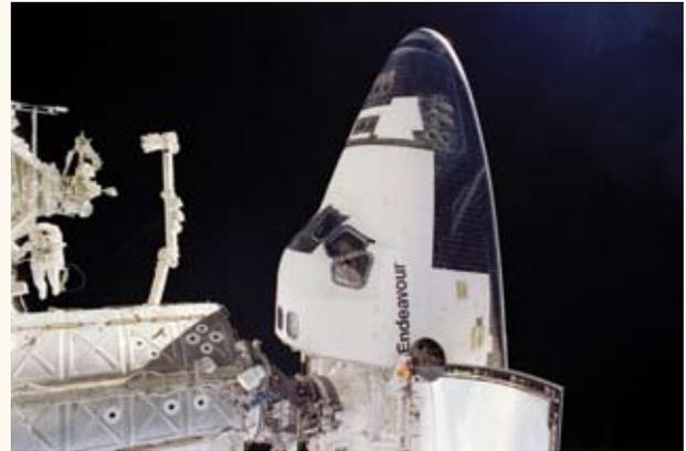
*Orbiter primary thrusters (three primary thrusters are visible closest to the nose cap on Endeavour)*
