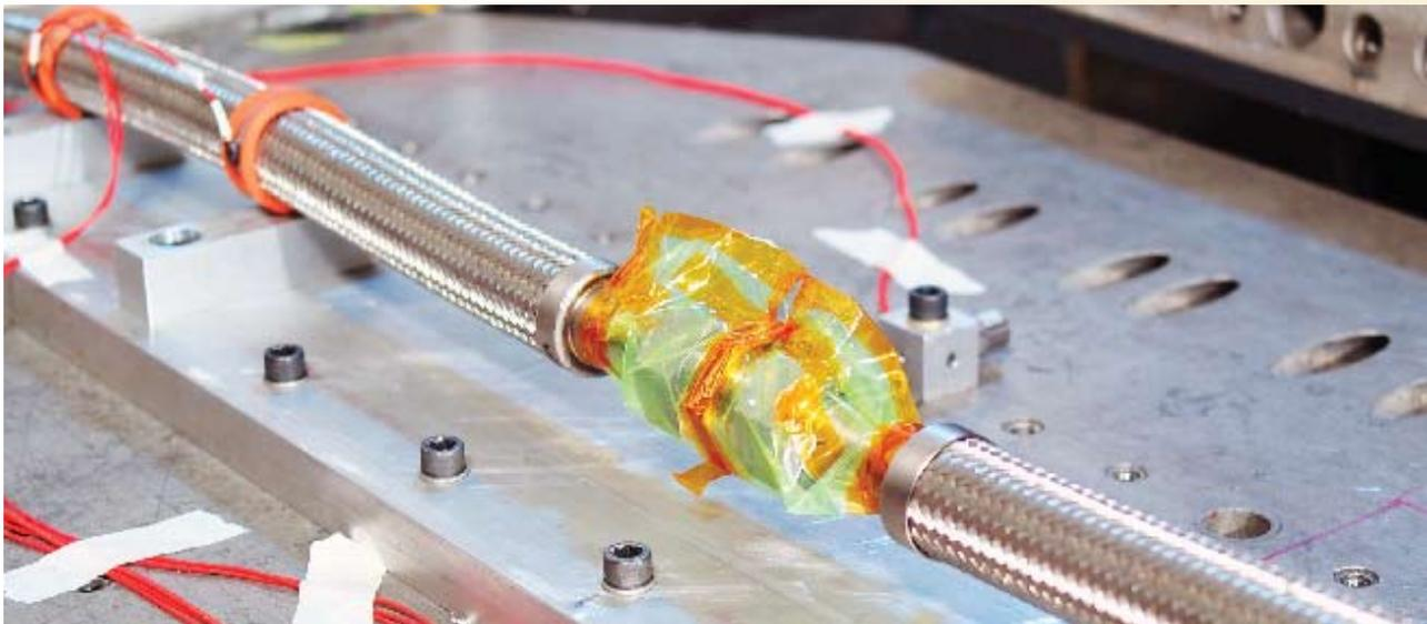
*AN fitting being prepared for helium leak test*
