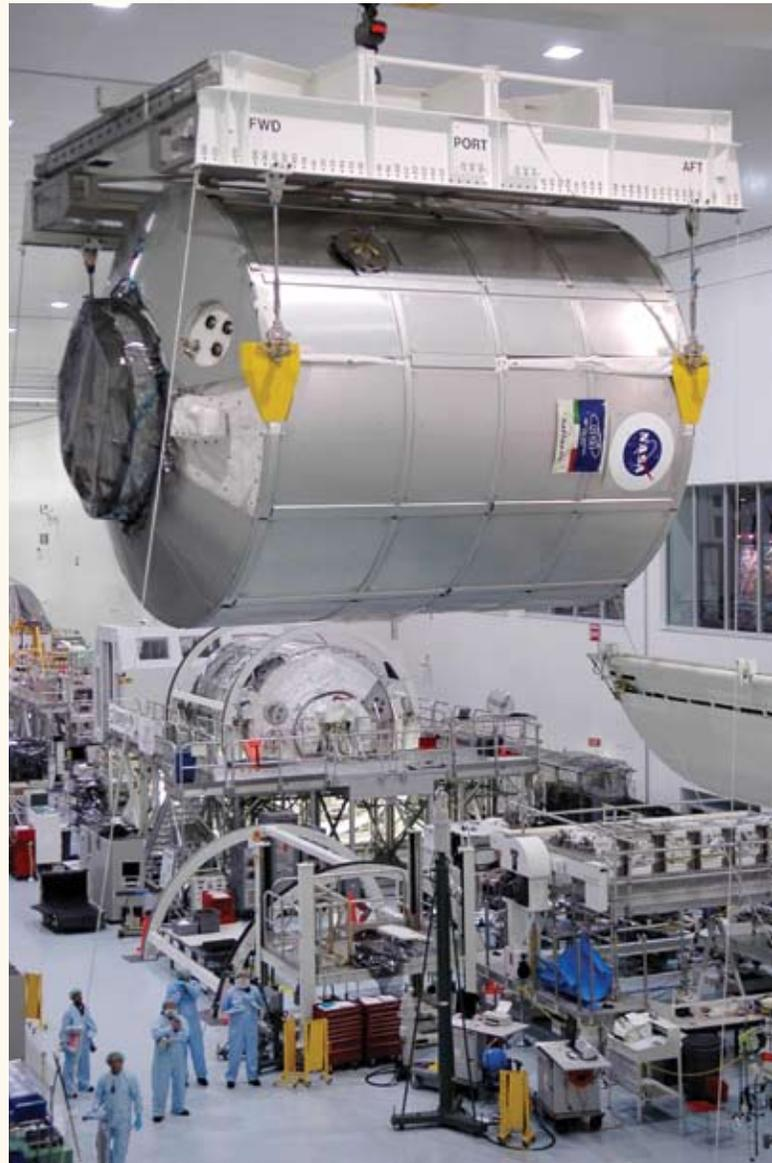
*Multi-purpose logistics module in the Space Station Processing Facility at Kennedy Space Center*
