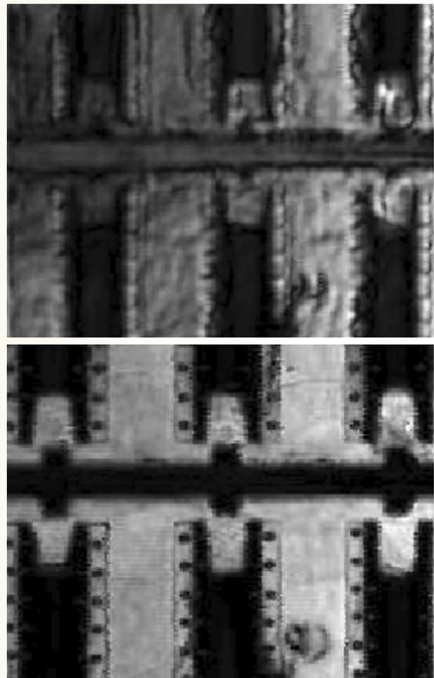
*Terahertz imaging of spray-on foam insulation
