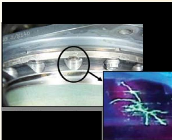
*Typical counter bore cracks visible under UV light with dye penetrant*
