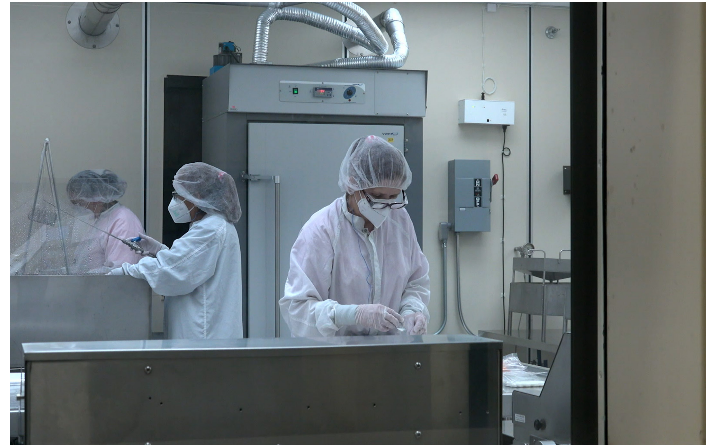
Johnson's Precision Cleaning Lab is necessary for removing oil and grease from spaceflight and ground support equipment to prevent rust and corrosion.
