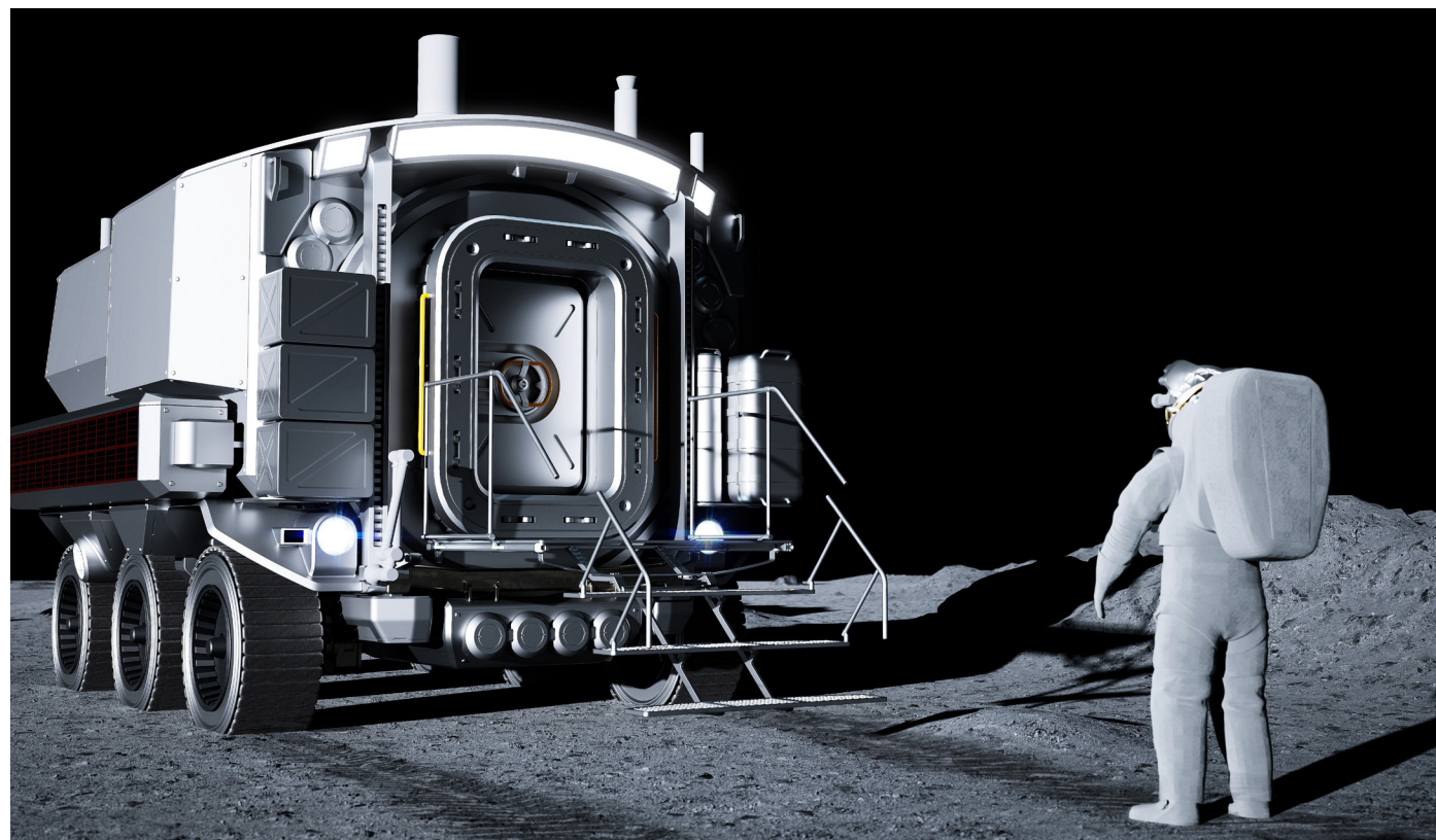
A concept image of the back of a pressurized rover on the surface of the Moon with the airlock in view. Image Credit: JAXA/Toyota
