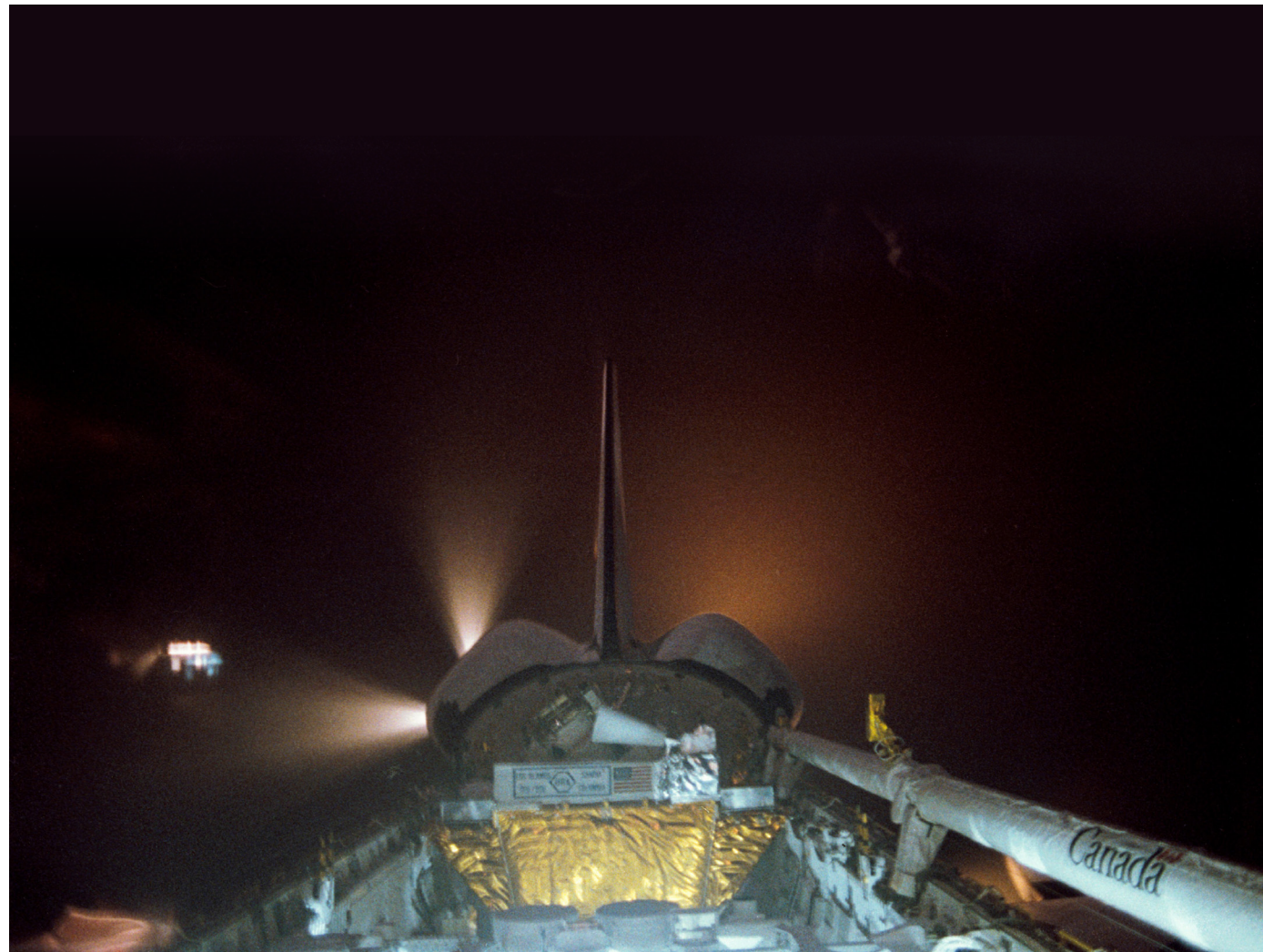
During its valve study, the NESC looked at past and present NASA programs in its search for common threads among valve failures. This included the Space Shuttle. Pictured here, the Space Shuttle Discovery fires reaction control subsystem (RCS) thrusters as seen from inside the crew cabin.
