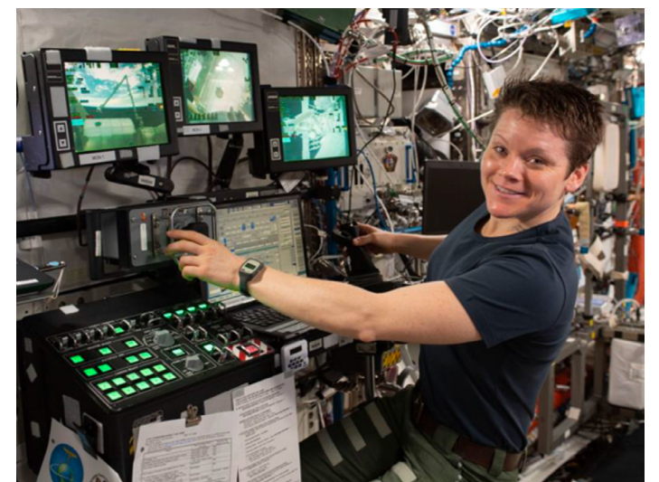
Figure 3. Astronaut Anne McClain using the Space Station Remote Manipulator System on ISS.
