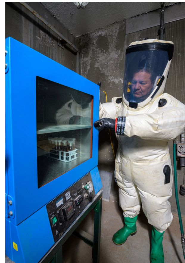
A technician at White Sands Test Facility removes test coupons from ovens during a coupon-exposure study.
