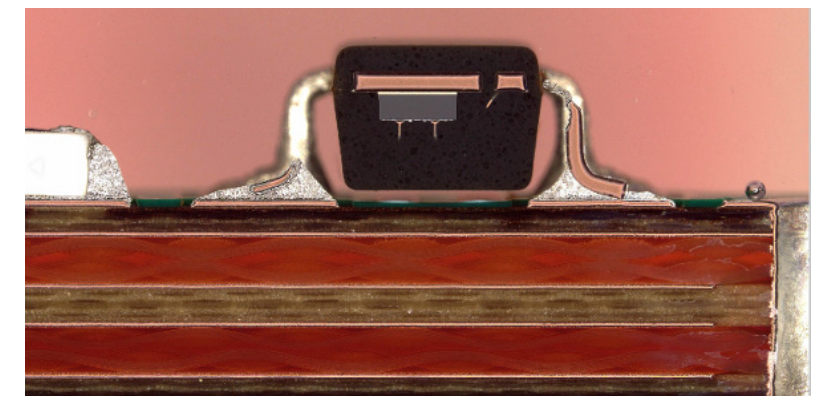
A public-facing database was created using cross-section images from the original NESc Cu Wire Bond Assessment and this follow-on work.
