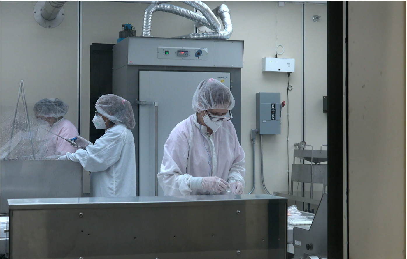
Johnson's Precision Cleaning Lab is necessary for removing oil and grease from spaceflight and ground support equipment to prevent rust and corrosion.
