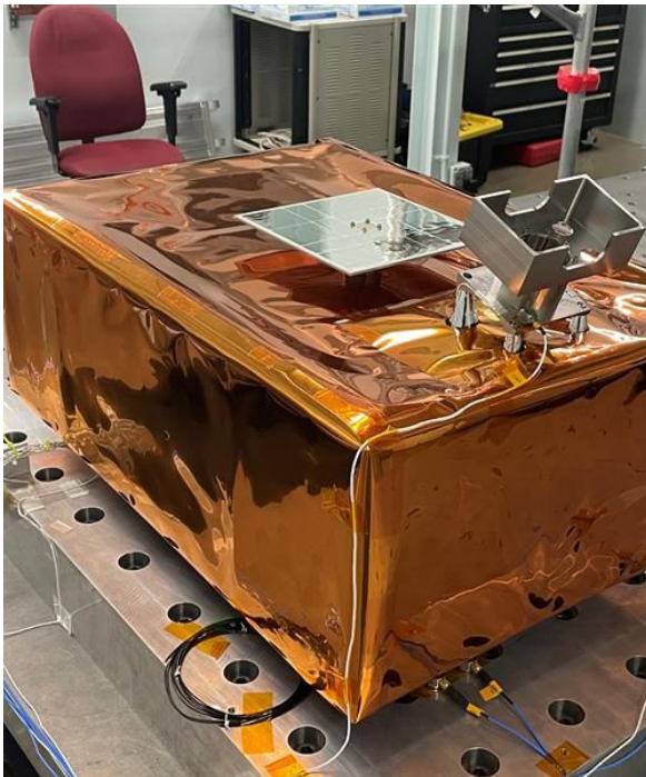
LEMS is a compact suite of seismometers, about the size of a carry-on suitcase, designed to continuously monitor the Moon’s surface for ground movement caused by moonquakes. Both meteoroid impacts and a shrinking and cooling moon cause the lunar surface and subsurface to shake.
