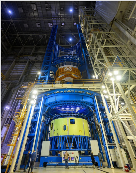
NASA's Friction Stir Welding lab resides inside NASA's Michoud Vertical Assembly Center in New Orleans and is being used to join major components of the SLS rocket.
