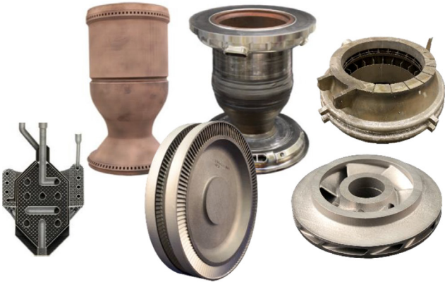
AM enables complex designs that were previously impractical or impossible to manufacture, but some parts will be challenging to reliably inspect per fracture control requirements.
