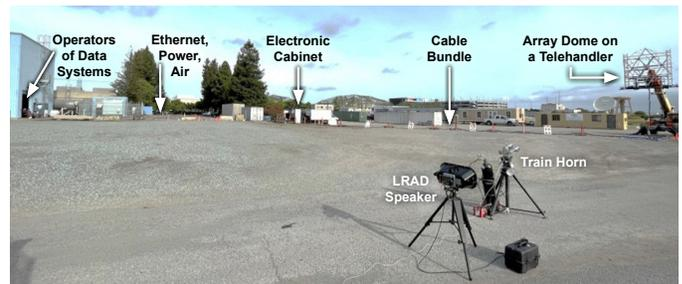
Figure 2. Setup for the outdoor test using a train horn and a long-range acoustic device (LRAD) speaker. The MPA was raised to test heights by a Telehandler.
