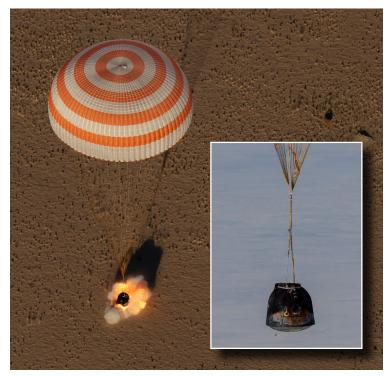
Soyuz decent module landing (inset) and firing of soft-landing rockets to reduce landing loads
