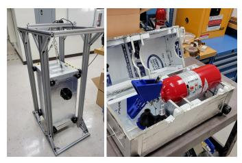
Figure 5. (left) PFE test stand for model validation. Design prevents directional load effects to enable accurate mass measurement during PFE discharge. Figure 6. (right) Insulated PFE housing and remote discharge control allows for accurate, real-time thermal measurements during validation testing.
