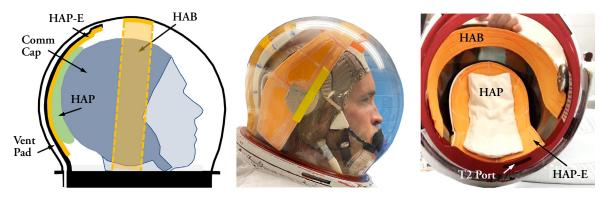
Figure 2. Water mitigation strategy for the ISS helmet: a) sketch of HAP, HAP-E, and HAB, b) side view of early prototype, c) bottom view of early prototype.
