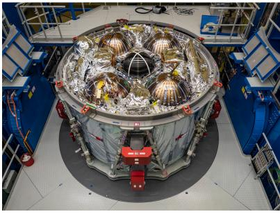
COPVs are used extensively in the Orion spacecraft service module.
