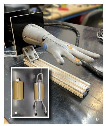
Figure 8. A) Mandrel used in cut testing as designed for ambient testing (left) and cryogenic testing (right). Flow channels allow for liquid nitrogen flow to cool the material sample to cryogenic temperatures. B) Prototype of Thermetrics, LLC custom manikin hand for spacesuit glove thermal testing.
