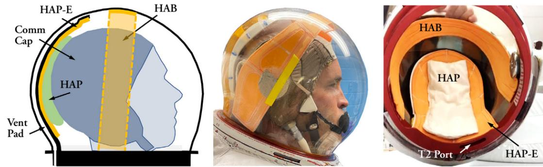
Figure 2. Water mitigation strategy for the ISS helmet: a) sketch of HAP, HAP-E, and HAB, b) side view of early prototype, c) bottom view of early prototype.
