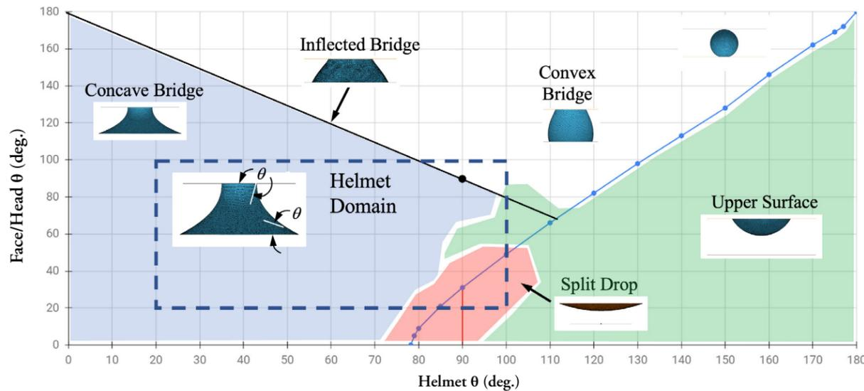
Figure 1. Map of predicted water formations within a helmet as a function of face/head and helmet contact angles. Dashed rectangle indicates the expected domain of the ISS helmet with no water mitigations.
