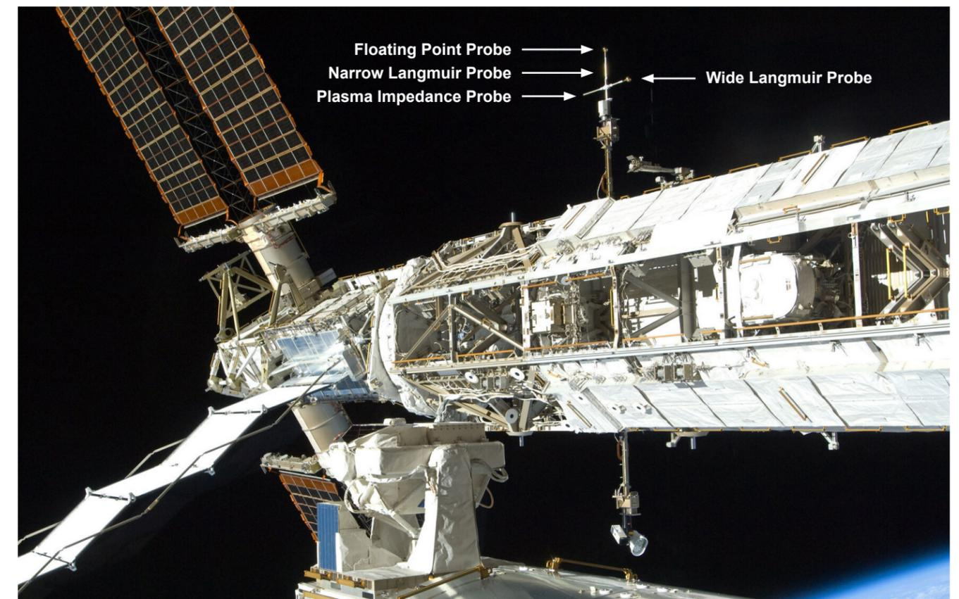
FPMU mounted to an ISS truss.
