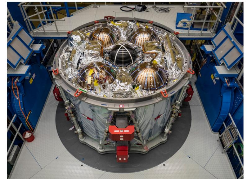
COPVs are used extensively in the Orion spacecraft service module.
