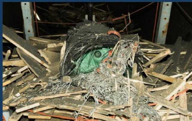
Results of a failure test. COPVs contain high pressure gases or fluids that can have tremendous explosive energy.
