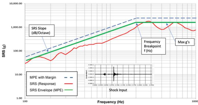
An example shock response spectrum (SRS) obtained from a mechanical shock separation system, indicating a broad signature is produced by pyro devices.
