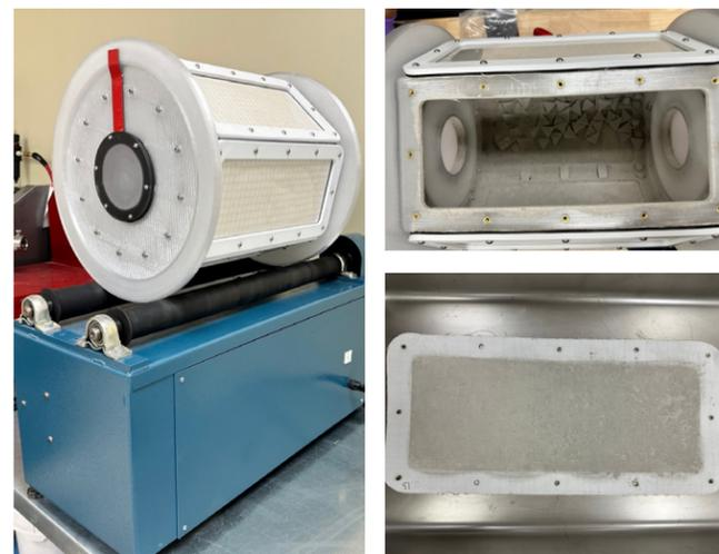
Figure 7. Hardware used in the tumble test method. Tumbler apparatus (left). Tumbler with panel removed to show lunar regolith simulant and commercially available tumbler media (top right). Tumbler panel showing lunar regolith simulant (bottom right).
