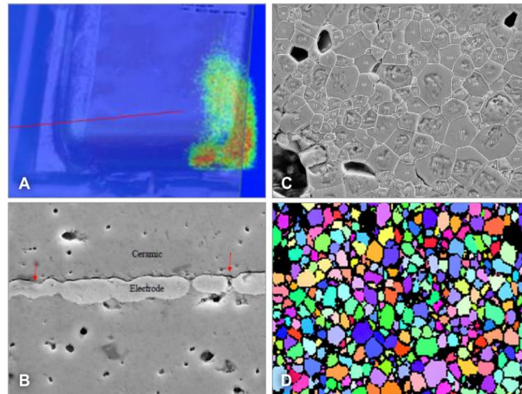
(A) Infrared image showing hot spot during powered test. (B) Electron microscope image showing delamination along the electrode plate associated with a crack (red arrows), which correlates with the IR region identified in A. (C) Manual tracing of grains (dark areas) on a scanning electron microscope image. (D) EBDS image. ImageJ software can analyze the EBDS image and provide statistics of colored grain regions to dark void regions.
