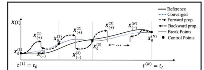
Figure 2. Multiple-shooting algorithm, utilizing strategic control points and a forward-backward propagation scheme.
