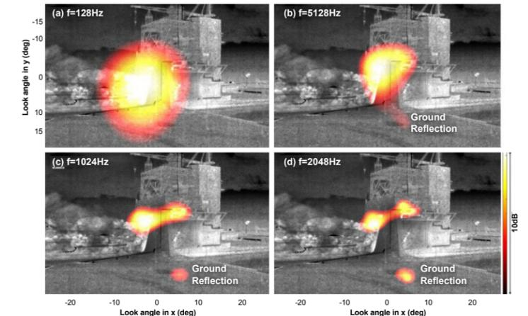
Figure 5. Noise sources identified at the indicated third-octave center frequencies using functional-orthogonal beamform.
