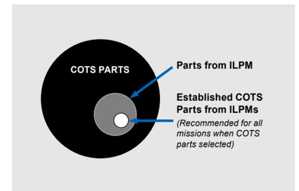
Established COTS parts are a subset of parts from an ILPM. An ILPM is a subset of COTS manufacturers.
