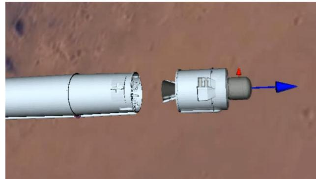
Frame of the Mars Ascent Vehicle second stage separation dynamics from an M&S animation.
