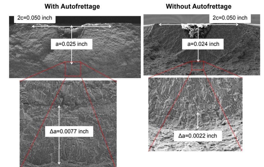
Figure 2. Fracture surfaces from two identical tests showing crack growth ( $\Delta a$ ), with and without an initial autofrettage cycle.
