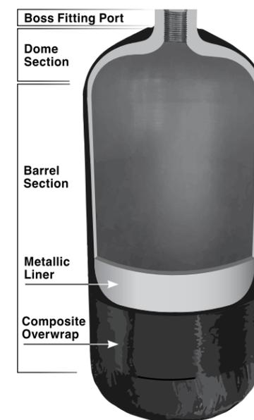
Figure 1. Illustration of COPV major components.
