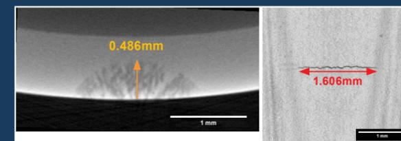
Computed tomography scan of a metallic liner detecting a part-through crack.
