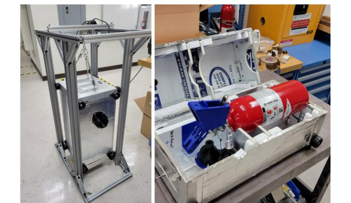
Figure 5. (left) PFE test stand for model validation. Design prevents directional load effects to enable accurate mass measurement during PFE discharge. Figure 6. (right) Insulated PFE housing and remote discharge control allows for accurate, real-time thermal measurements during validation testing.
