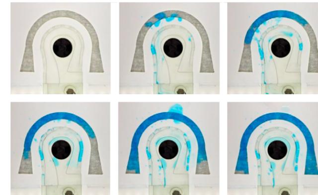
Figure 3. HAB ground validation testing under trickle water flow conditions.
