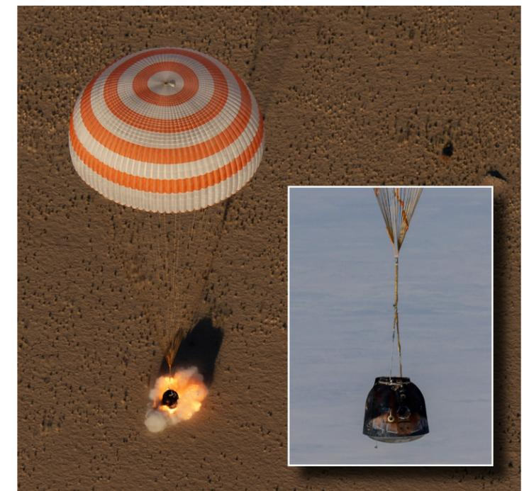
Soyuz descent module landing (inset) and firing of soft-landing rockets to reduce landing loads.
