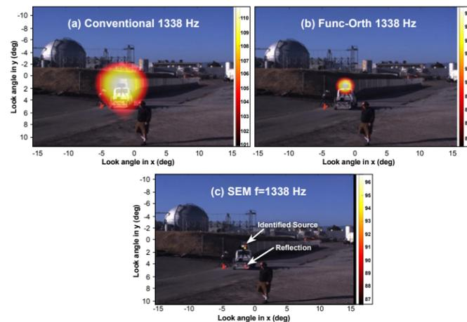
Figure 3. Comparison between different beamform schemes at a fixed  $f=1338$  Hz with array center 100 ft. horizontal and 10 ft. above LRAD speaker.
