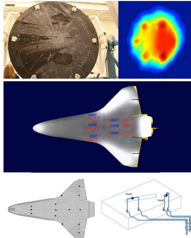
(Top) Orion EFT-1 heatshield included embedded TCs. Colorized infrared (IR) reentry image data used to correlate temperature with TC readings. (Middle) IR image of STS-115 overlaid on orbiter CAD model showing location of TCs. (Bottom) Location of TCs on Endeavor and TC configurations for reentry temperature measurement experiment on STS-134.
