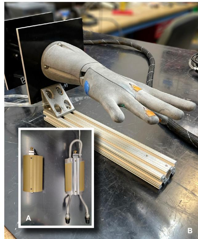
Figure 8. A) Mandrel used in cut testing as designed for ambient testing (left) and cryogenic testing (right). Flow channels allow for liquid nitrogen flow to cool the material sample to cryogenic temperatures. B) Prototype of Thermetrics, LLC custom manikin hand for spacesuit glove thermal testing.
