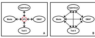
Figure 1. A) Interoperability between flight mechanics tools using standardized trajectory structures. B) Traditional specific tool-to-tool interface design.
