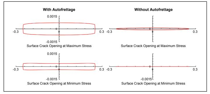
Figure 3. Abaqus finite element analysis of crack growth with and without an autofrettage cycle. Y-axis indicates crack opening displacement and x-axis indicates crack length.
