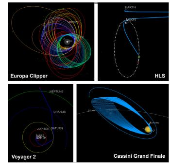
Figure 3. Future and flown missions reconstructions using Copernicus (Europa Clipper, Cassini) and Monte (HLS, Voyager 2) from SPK obtained from the Horizons System database at https://ssd.jpl.nasa.gov/horizons/.
