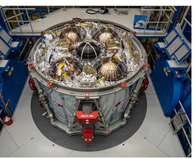
COPVs are used extensively in the Orion spacecraft service module.
