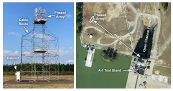
Figure 4. Scaffold system used to mount MPA and location of the arrav with respect to the SSC A-1 test stand. Right Image Credit: Google Maps
