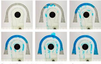
Figure 3. HAB ground validation testing under trickle water flow conditions.
