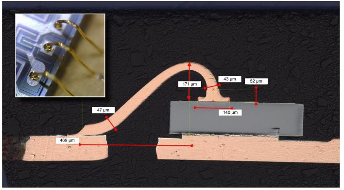
Example of gold wire bonds. Wire bonds transfer electrical signals to/from an integrated circuit's external terminals and the internal microcircuits.
