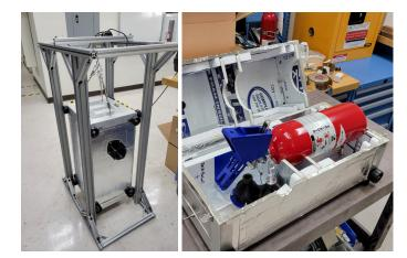
Figure 5. (left) PFE test stand for model validation. Design prevents directional load effects to enable accurate mass measurement during PFE discharge. Figure 6. (right) Insulated PFE housing and remote discharge control allows for accurate, real-time thermal measurements during validation testing.
