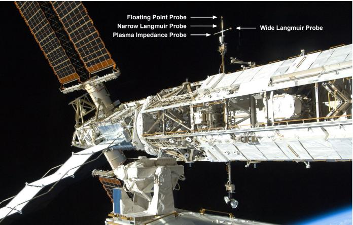
FPMU mounted to an ISS truss
