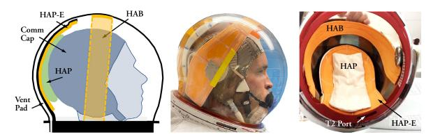
Figure 2. Water mitigation strategy for the ISS helmet: a) sketch of HAP, HAP-E, and HAB, b) side view of early prototype, c) bottom view of early prototype.
