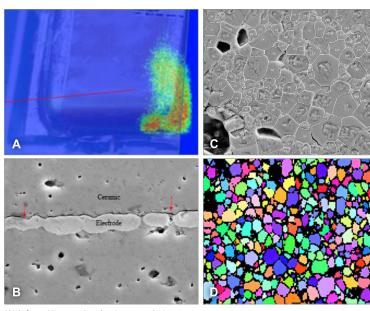
(A) Infrared image showing hot spot during powered test. (B) Electron microscope image showing delamination along the electrode plate associated with a crack (red arrows), which correlates with the IR region identified in A.
