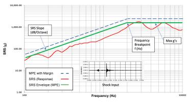
An example shock response spectrum (SRS) obtained from a mechanical shock separation system, indicating a broad signature is produced by pyro devices.
