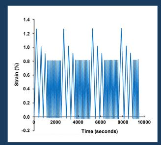
Representative loading spectrum for an elastically responding COPV liner with an initial elastic-plastic cycle.
