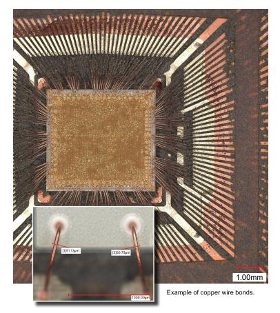
the widest range of NASA mission conditions. Based on results for the parts tested, they found the reliability of copper wire bonds to be comparable to gold bonds. The team also developed screening and lot acceptance testing guidelines for evaluating copper-wire bonds in plastic parts for a range of NASA flight conditions and mission risk classifications. *This work was performed by LaRC, JPL, GSFC, JSC, KSC, WFF, MSFC, and OSMA.* <u>NASA/TM 20230014536</u>.
