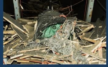
Results of a failure test. COPVs contain high pressure gases or fluids that can have tremendous explosive energy.
