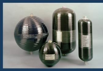
A COPV consists of a metallic liner with an exterior composite wrap. The composite provides strength, and the liner contains the compressed fluid or gas.
