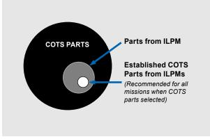
Established COTS parts are a subset of parts from an ILPM. An ILPM is a subset of COTS manufacturers
