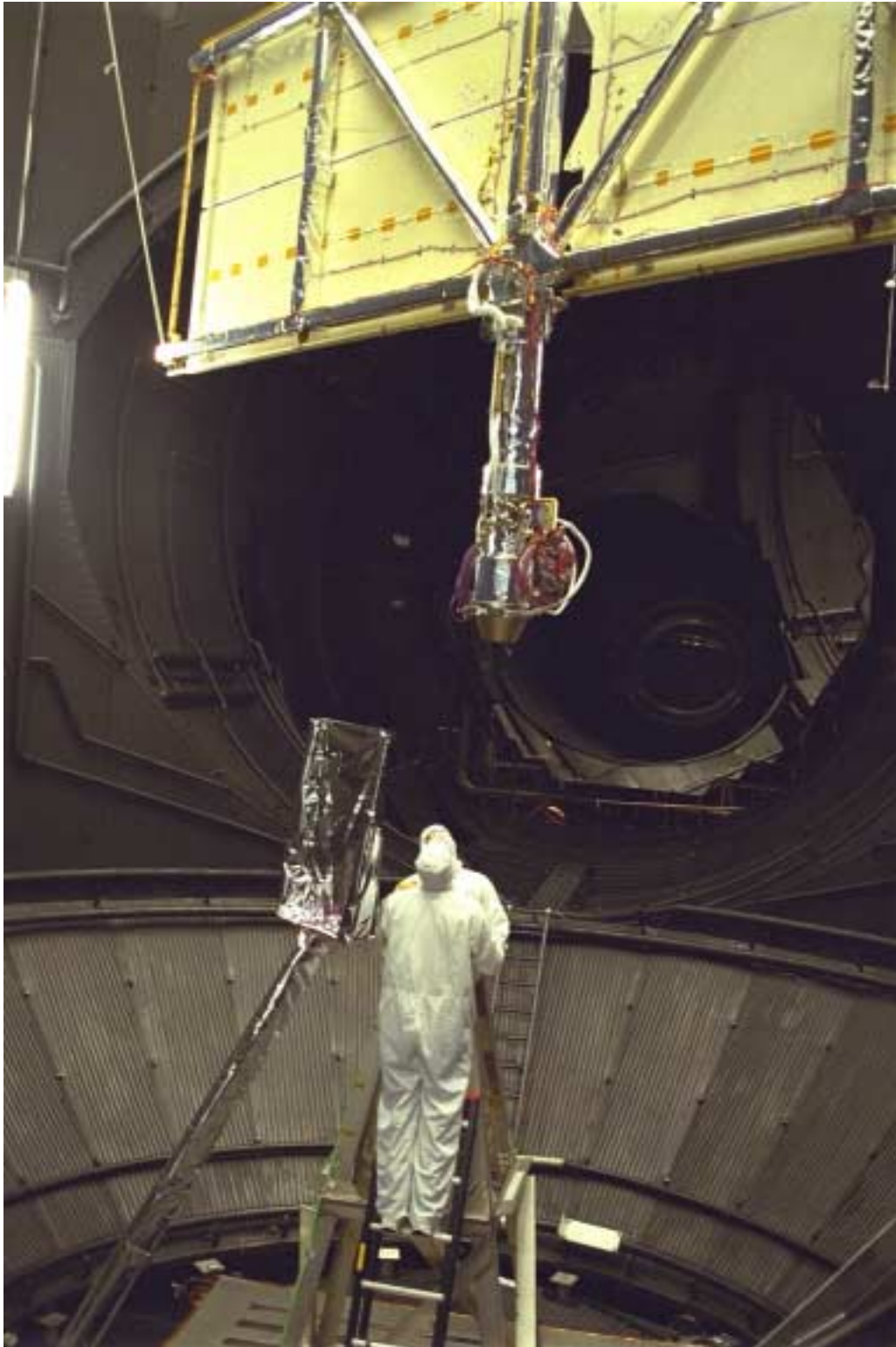
One wing of Solar Array 3 is lowered into a chamber for testing. The new rigid arrays will produce 20 percent more power.
