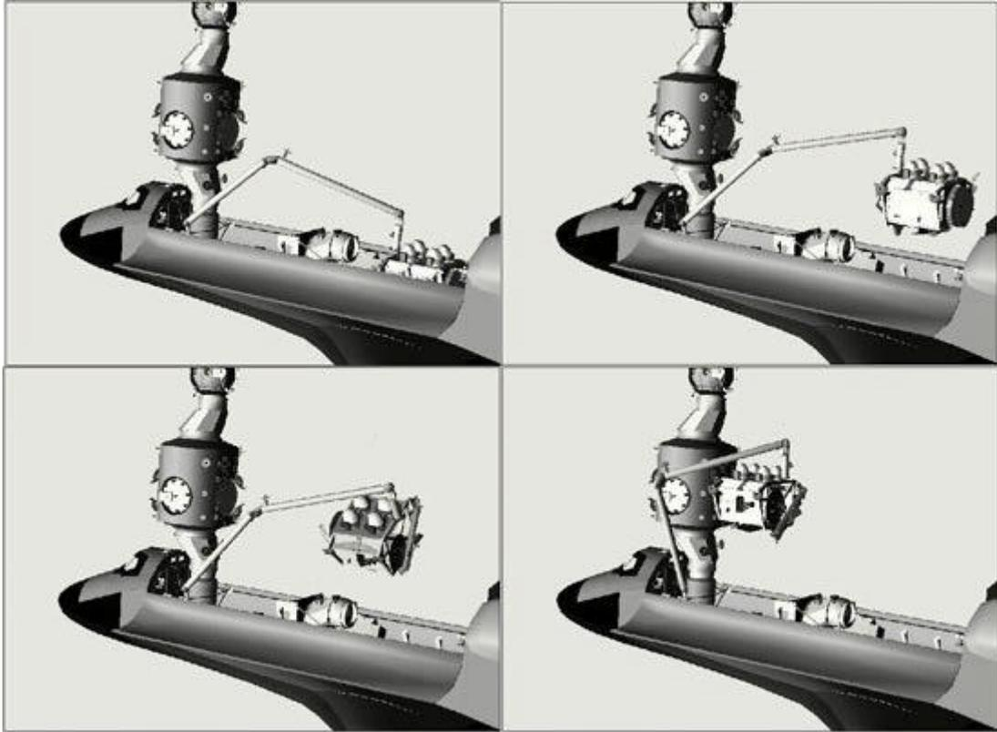
*Figure 1. Z1 Installation*
