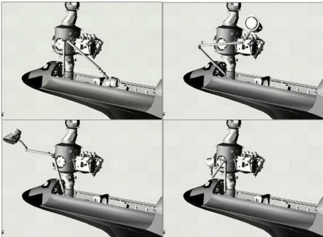
*Figure 2. PMA-3 Installation*
