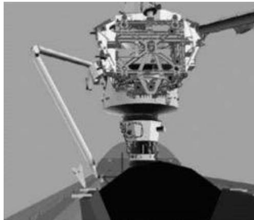
*Figure 10. PMA-3- to Node 1 Umbilical Connection*
