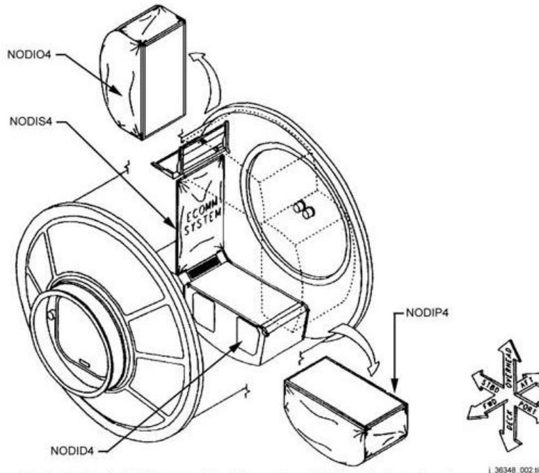
*Node 1 On-Orbit Stowage Configuration (Soft Racks Deployed)*
