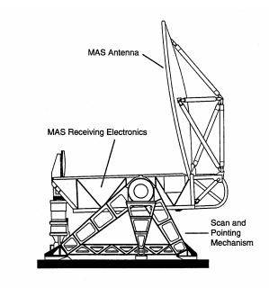
Millimeter-Wave Atmospheric Sounder (MAS)
