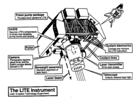
Laser light, directed toward Earth, will bounce off of thin clouds, dust particles and the surface of the Earth -- LITE's telescope receiver will "catch" that reflected light.
