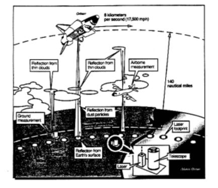
Laser light from the shuttle contacts thin clouds, dust particles and the Earth's surface, and a reflection is bounced back to LITE's telescope.
