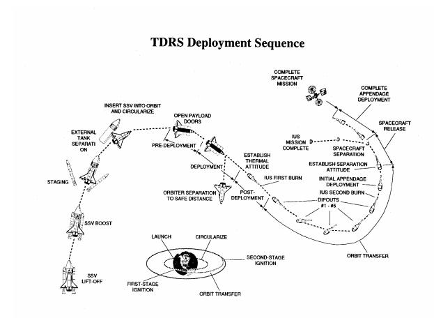
Forward payload restraints are released and the aft frame of the airborne support equipment tilts the IUS/TDRS to 29 degrees. This extends the TDRS into space just outside the orbiter payload bay, allowing direct communication with Earth during systems checkout. The orbiter then is maneuvered to the deployment attitude. If a problem develops within the spacecraft or IUS, the IUS and its payload can be restowed.
