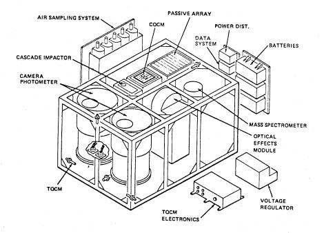
With the monitor instrumentation, contaminant sources are identified for possible elimination. The experiment provides data on the interaction of the induced and natural environments, and provides critical data for planning of future Shuttle payloads.
