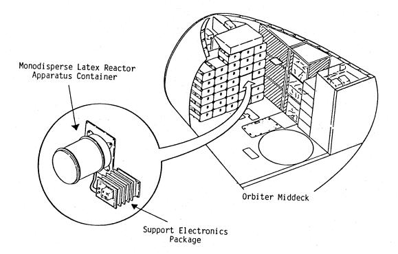
On Earth, these beads can be produced only up to about three microns and still be monodisperse. The experiment which will be flown on a total of four flights will help determine if much larger (larger than 20 microns) monodisperse beads can be produced practically and economically in space.
