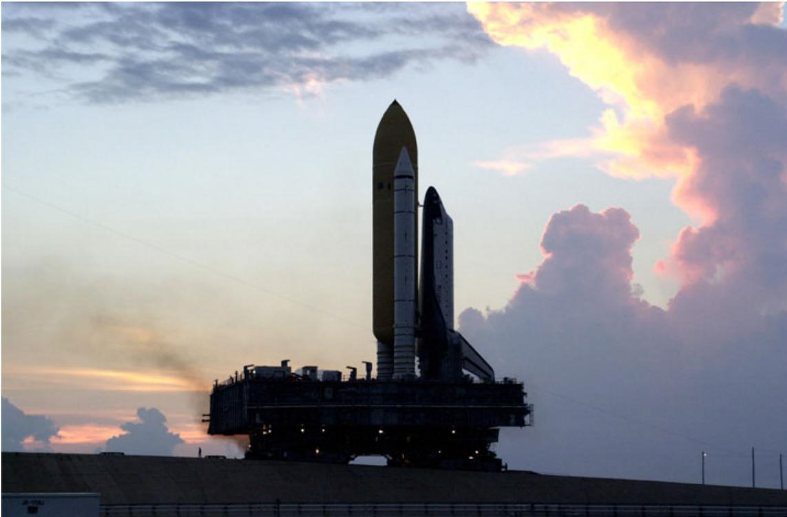
***Space shuttle Endeavour is rolled to the Kennedy Space Center Launch Pad 39A on top of the Mobile Launch Platform, moved by the crawler-transporter underneath.***
