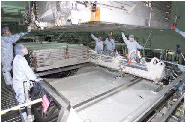
**Boeing technicians install a radiator on the Port One (P1) Truss inside the Kennedy Space Center, Fla., Space Station Processing Facility during summer 2002. The radiator will be used to control the temperature of the International Space Station's electronics.**
