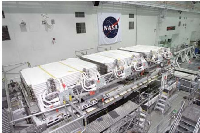
***The Port One (P1) Truss for the International Space Station sits inside the Kennedy Space Center, Fla., Space Station Processing Facility during June 2002. The radiator assembly (covered by white thermal blankets) can be seen on top of the truss. Space shuttle Endeavour will deliver P1 during mission STS-113.***
