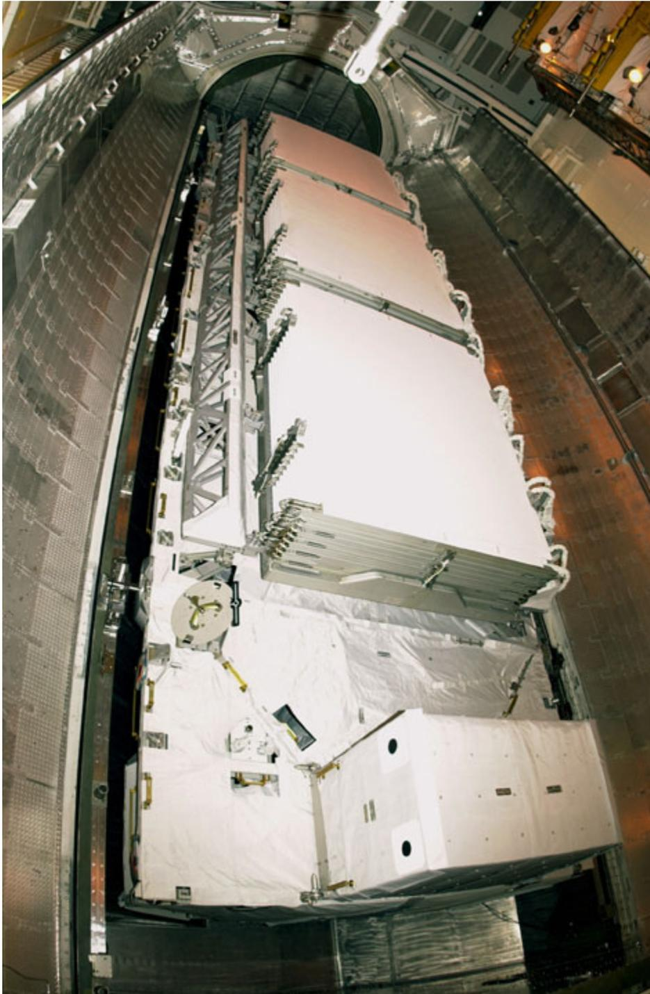
***At Launch Complex 39A, the payload canister doors are open to reveal the P1 Truss before transfer to the Payload Changeout Room.***
