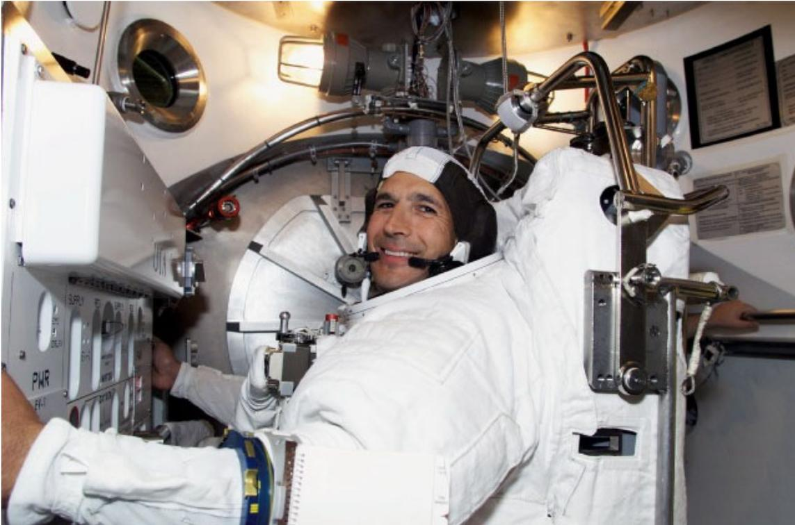
***Astronaut John B. Herrington, STS-113 mission specialist, participates in an Extravehicular Mobility Unit (EMU) fit check in a Space Station Airlock Test Article (SSATA) in the Crew Systems Laboratory at the Johnson Space Center (JSC).***
