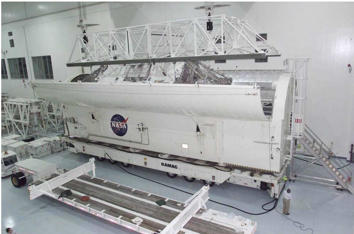
The S0 truss is lifted into its transport canister at the Kennedy Space Center.
