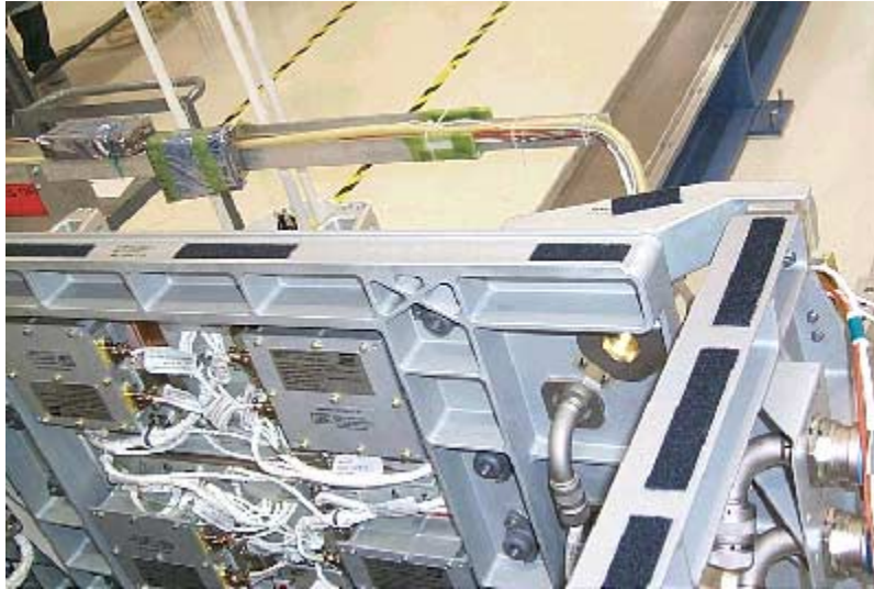
The Amplifier Orbital Replacement Unit buffers and amplifies data signals between the Mobile Transporter and Trailing Umbilical System and between the Mobile Remote Servicer and Trailing Umbilical System.
