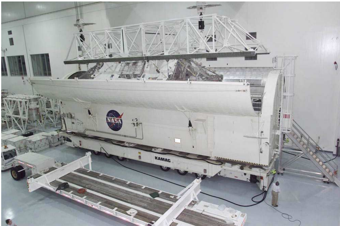
The S0 truss is lowered into its transport canister at the Kennedy Space Center.
