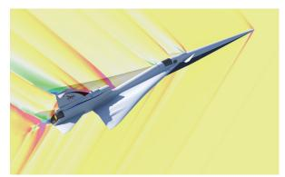
Computer simulation showing how shock waves move away from the X-59 as it flies faster than sound. The pattern is different from the way shock waves from a conventional supersonic aircraft come together to produce a sonic boom. Instead, the X-59 will produce a quieter sonic thump. Credit: NASA
