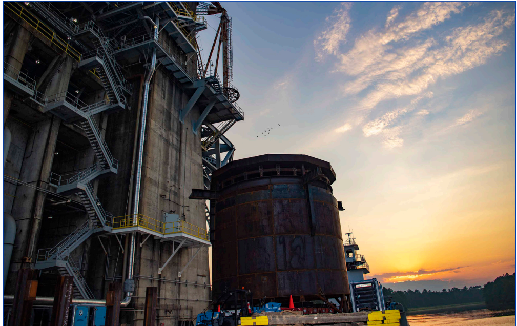
Sunrise offers a perfect frame for the interstage simulator component following its arrival at the B-2 Test Stand at NASA's Stennis Space Center on Sept. 21, 2022. Stennis will use the unit during testing of the Exploration Upper Stage for NASA's Space Launch System rocket. Photo credit: (NASA/Danny Nowlin)
