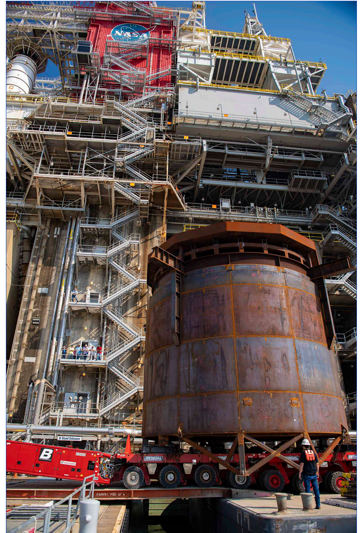
for NASA's Space Launch System rocket. (Right photo) The close up view of the interstage simulator component shows how massive the test component is in comparison to the B-2 Test Stand and nearby workers at the stand. Photo credit: (NASA/Danny Nowlin)
