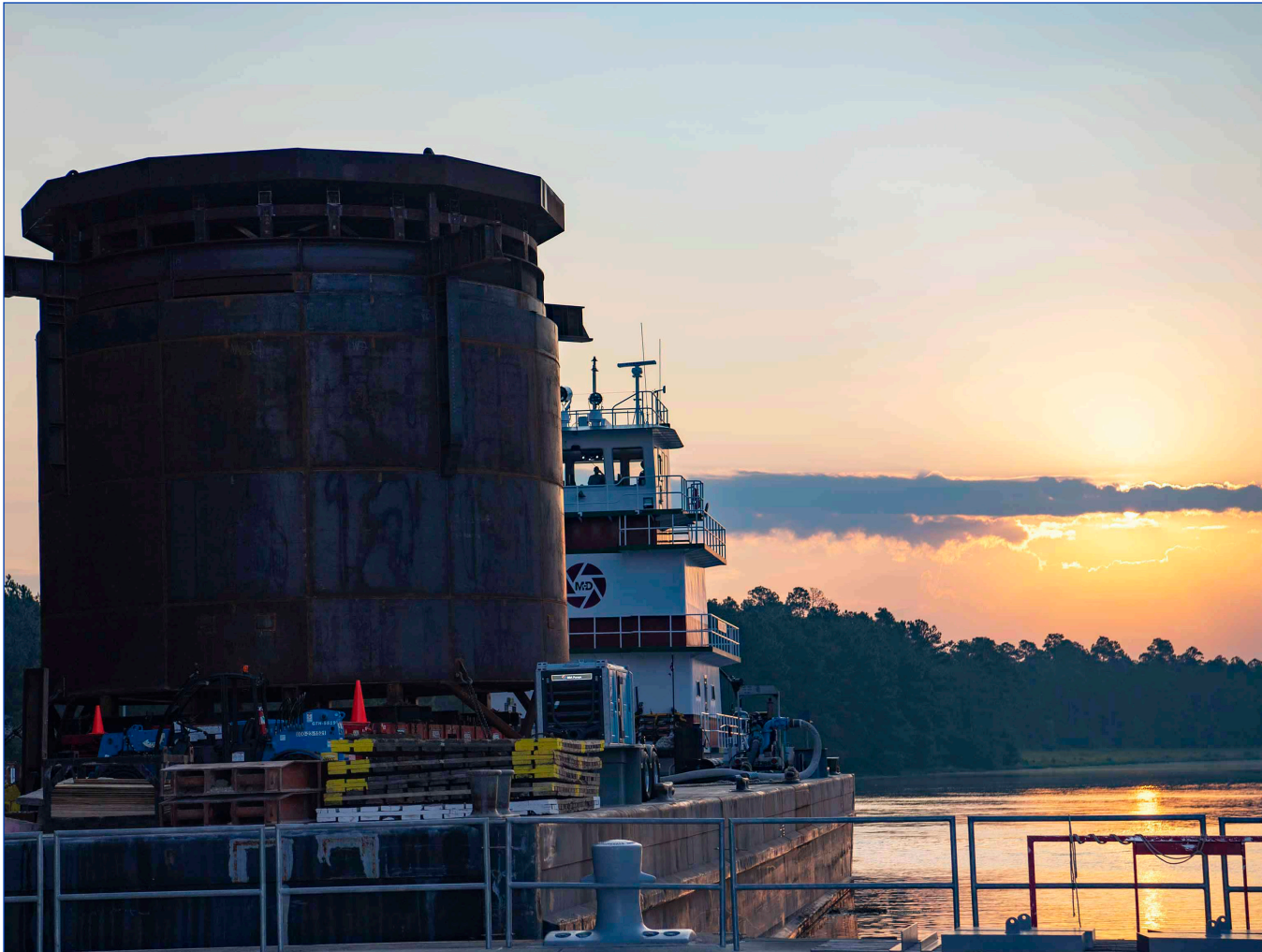
The interstage simulator component to be used during Exploration Upper Stage testing for the Space Launch System rocket arrives at the B-2 Test Stand NASA's Stennis Space Center on Sept. 21, 2022. Photo credit: (NASA/Danny Nowlin)
