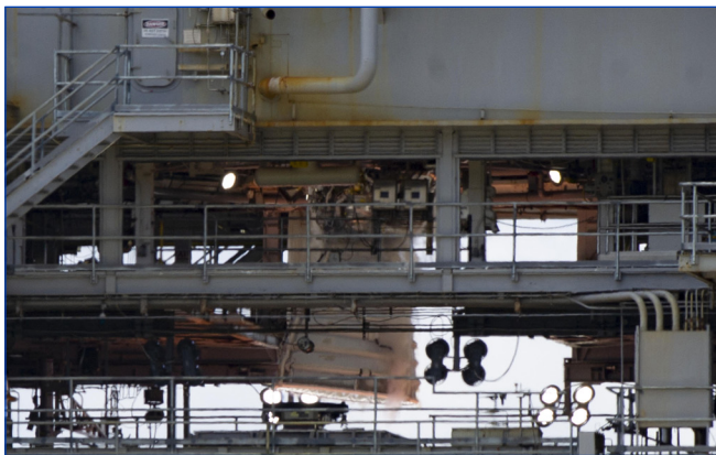
(Top photo) NASA conducts an RS-25 hot fire test on the Fred Haise Test Stand at NASA's Stennis Space Center in south Mississippi on April 26.
