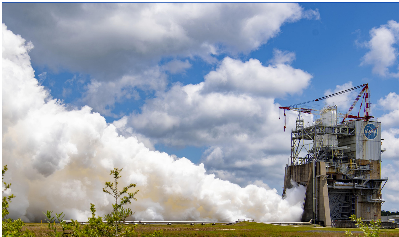
NASA conducts an RS-25 hot fire test on the Fred Haise Test Stand at NASA's Stennis Space Center in south Mississippi on April 26.
