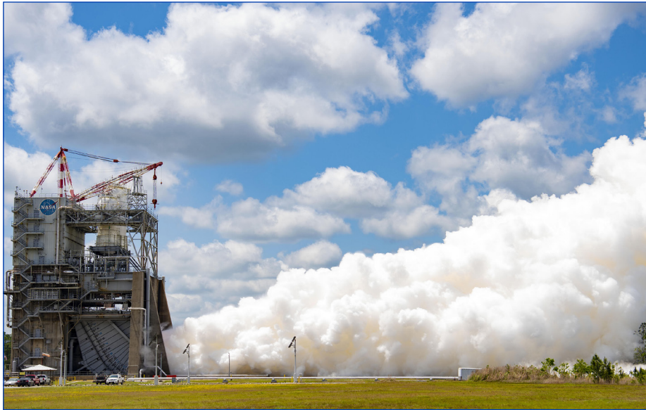
(Top photo) NASA conducts an RS-25 hot fire test on the Fred Haise Test Stand at NASA's Stennis Space Center in south Mississippi on April 26.
