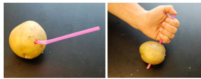
An open straw has equal pressure inside and out. It is not very rigid and will not go very far into the potato without buckling.
