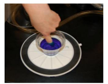
*Testing water temperature immediately after the water leaves the vacuum environment.*
