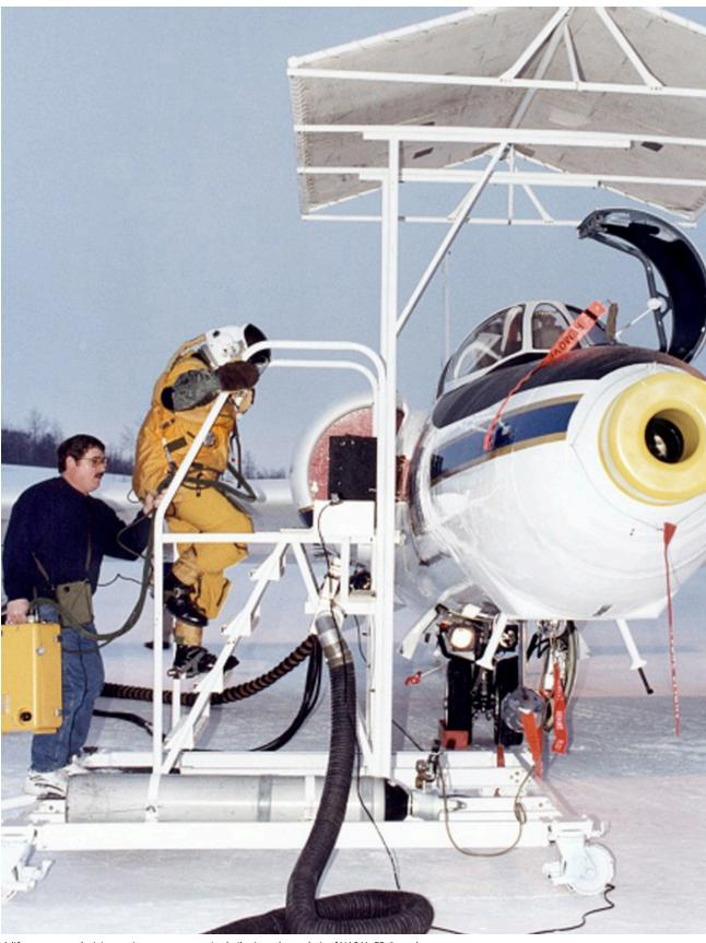
A life-support technician assists a pressure-suited pilot into the cockpit of NASA's ER-2 earth resources aircraft. (Image Credit: NASA, http://www.dfrc.nasa.gov/Gallery/Photo/ER-2/Small/EC00-0037-27.jpg)
