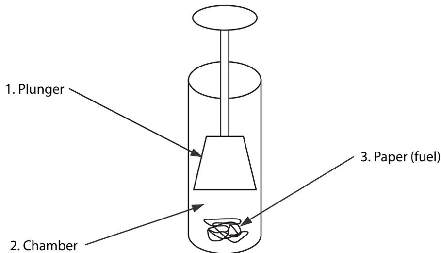
2. The Fire Syringe is much like the piston of a diesel engine. What is the fuel for a diesel engine's piston?
