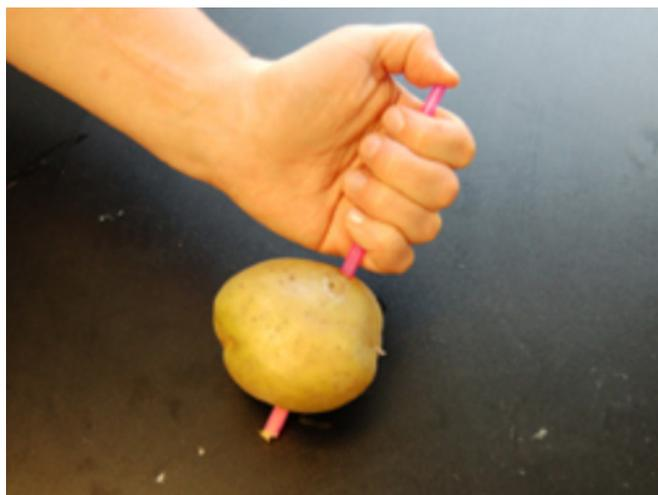
*When the end of the straw is blocked, pressure increases inside the straw as it is pushed into the potato, thus increasing the rigidity of the straw and preventing buckling.*
