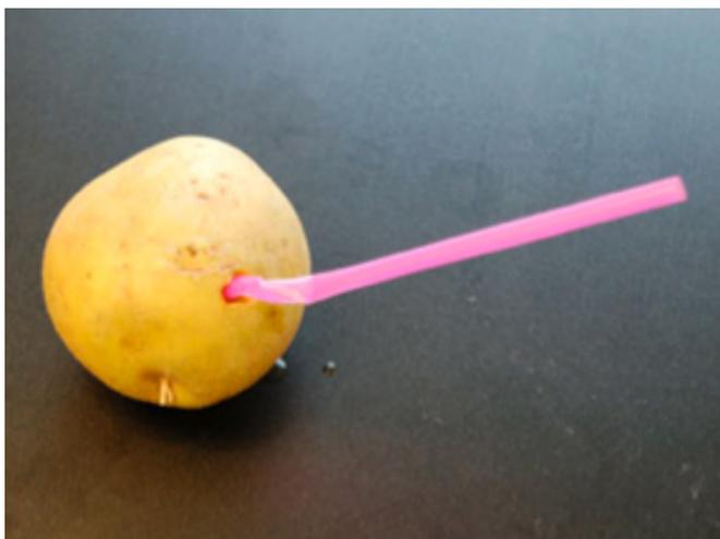
*An open straw has equal pressure inside and out. It is not very rigid and will not go very far into the potato without buckling.*
