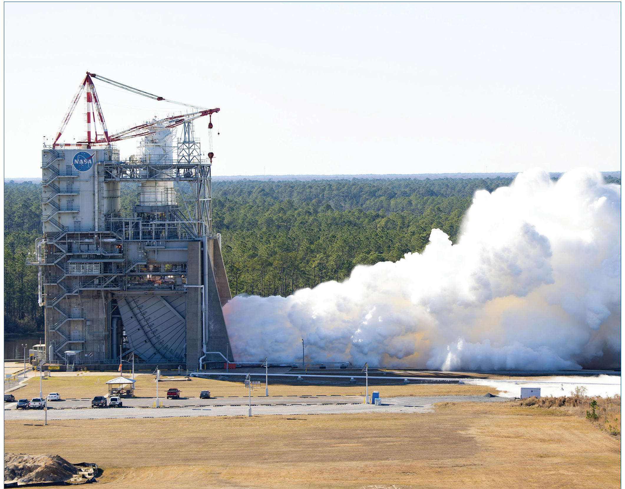
NASA conducted its second RS-25 engine hot fire test of 2022 on Feb. 8 on the Fred Haise Test Stand. Each test in the series provided valuable operational data to NASA's lead engines contractor, Aerojet Rocketdyne, on a variety of new
