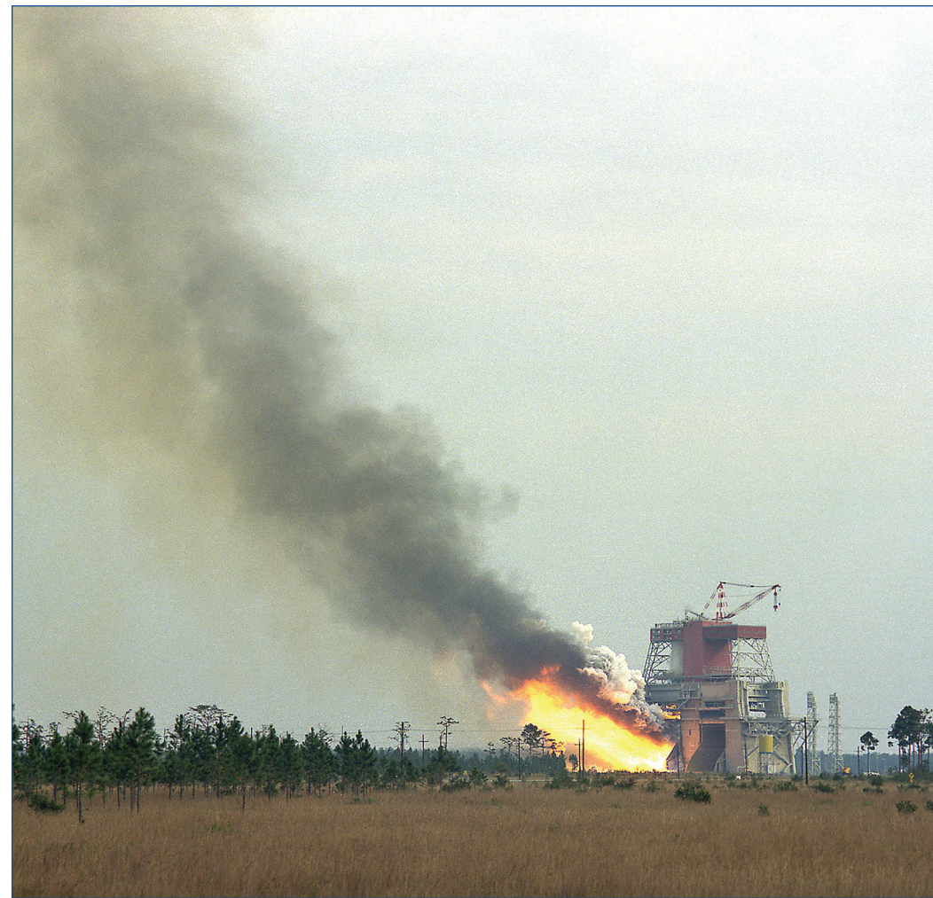
NASA conducts a hot fire test of the Saturn V S-IC-12 stage on the B-2 Test Stand at NASA's Stennis Space Center on Nov. 3, 1969. A little more than a year later, the unit fired again to launch the Apollo 17 mission to the Moon.
