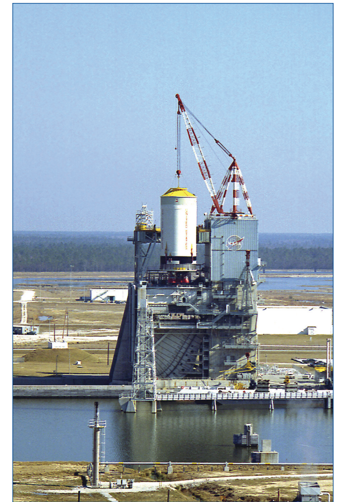
Teams at NASA's Stennis Space Center install the Saturn V S-II-12 stage on the A-2 Test Stand on Dec. 22, 1969, in preparation for hot fire testing prior to use on the Apollo 19 mission.
