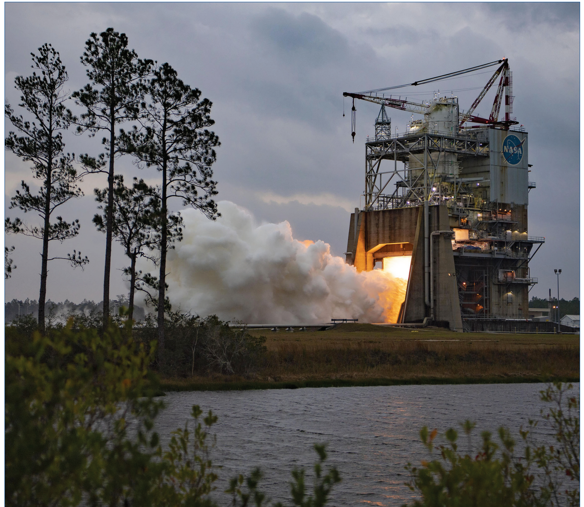
NASA conducts an RS-25 hot fire on the Fred Haise Test Stand at Stennis Space Center in south Mississippi on Dec. 14. Photo Credit: (NASA/Danny Nowlin)
