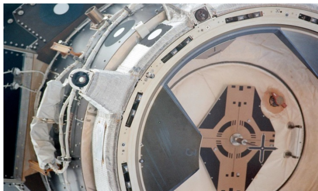
Docking target inside one of the docking adapters aboard the International Space Station.
