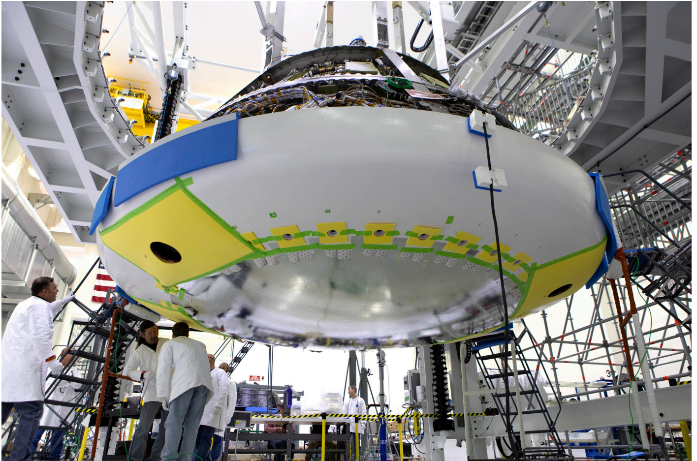
Installation of the heat shield on NASA's Orion spacecraft crew module at Kennedy Space Center in Florida on July 25, 2018. (NASA/Kim Shiflett)
