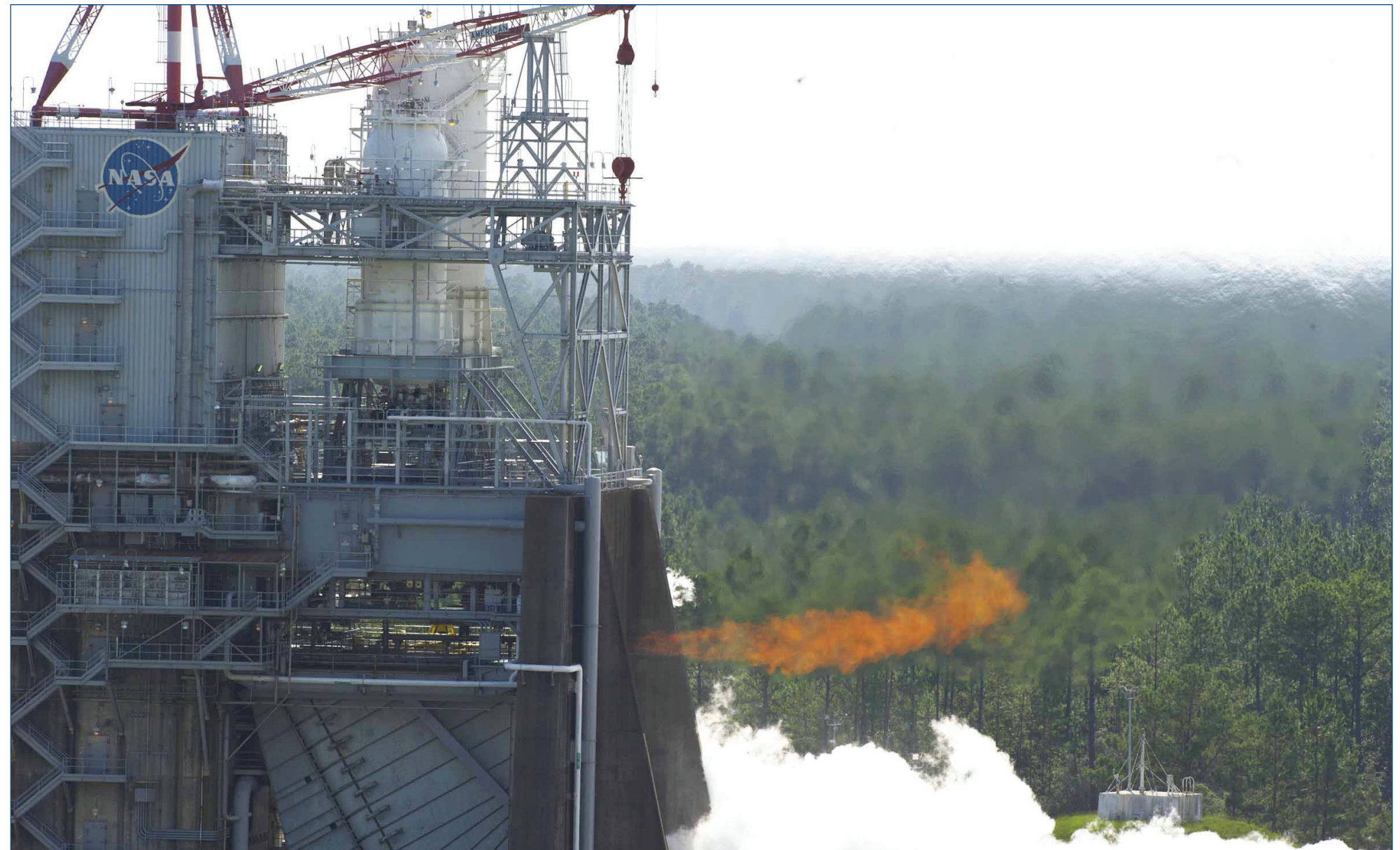
Operators conduct a record-setting hot fire of an upgraded J-2X powerpack on the Fred Haise Test Stand on July 24, 2012. The flame exiting the test stand through the discharge duct is from the combustion of the test article. The powerpack fired for 1,350 seconds, surpassing a previous record of 1,150 seconds established just six weeks earlier. The hot fire still stands as the longest-duration test ever conducted in the A Test Complex. Photo Credit: (NASA/Danny Nowlin)
