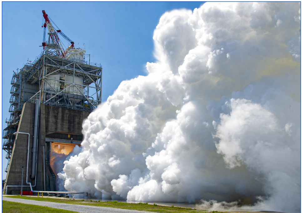
(Bottom photo) A mounted camera near the Fred Haise Test Stand shows the RS-25 certification engine test underway on April 5.
