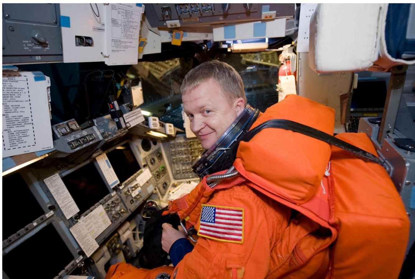
Attired in a training version of his shuttle launch and entry suit, NASA astronaut Eric Boe, STS-133 pilot, occupies the pilot's seat during a simulation exercise in the motion-base shuttle mission simulator in the Jake Garn Simulation and Training Facility at NASA's Johnson Space Center.
