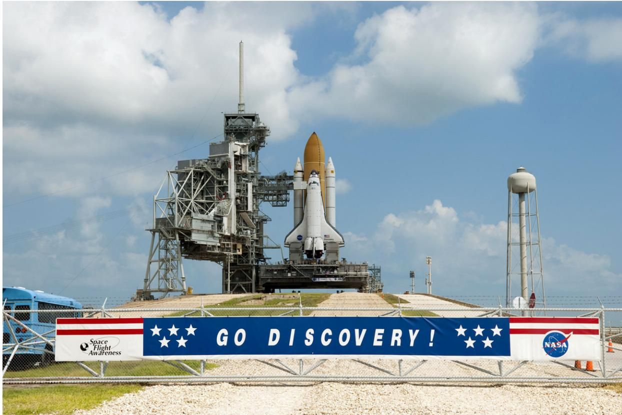
**At NASA’s Kennedy Space Center in Florida, space shuttle Discovery is poised for the STS-133 launch from Launch Pad 39A following the roughly six-hour journey, known as “rollout,” from the Vehicle Assembly Building to the pad. Image credit: NASA/Jim Grossmann**
