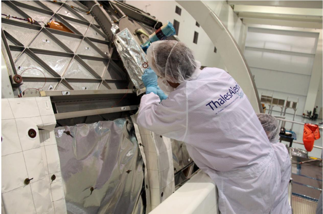
In the Space Station Processing Facility at NASA’s Kennedy Space Center in Florida, a technician installs multilayer insulation on the meteoroids and debris protective shield of the Permanent Multipurpose Module. The reflective silver mesh is Mylar, which is aluminized to protect hardware aboard the International Space Station from solar thermal radiation.
