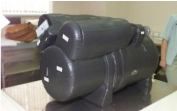
assembly is completely enclosed in thermal insulation. The PPA weighs 191 pounds with the ITCS fluid fill. It measures 29.64 inches by 18.63 inches by 17.75 inches. The PPAs are manufactured by Honeywell, Inc., Torrance, Calif.
