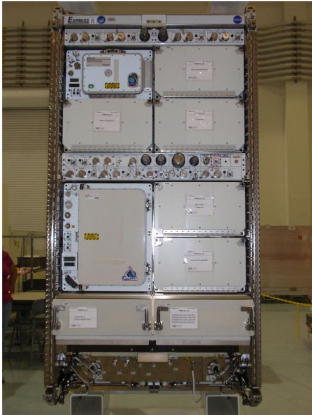
power, data, command and control, video, water cooling, air cooling, vacuum exhaust and nitrogen supply to payloads. Each Express rack is housed in an international standard payload rack (ISPR), a refrigerator-sized container that serves as the rack's exterior shell.
