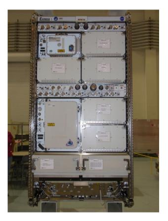
power, data, command and control, video, water cooling, air cooling, vacuum exhaust and nitrogen supply to payloads. Each Express rack is housed in an international standard payload rack (ISPR), a refrigerator-sized container that serves as the rack's exterior shell.
