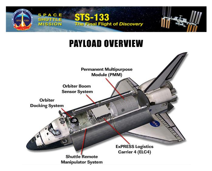
This graphic depicts the space shuttle Discovery's payload bay for STS-133, which includes the Permanent Multipurpose Module and the Express Logistics Carrier 4. The total payload weight, not counting the middeck, is 36,514 pounds.
