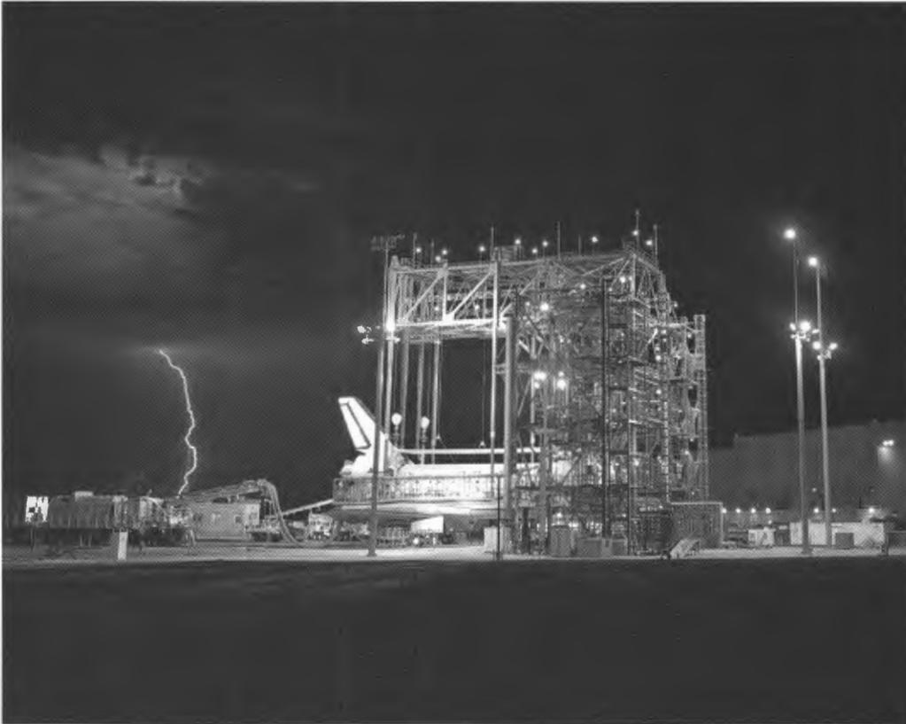
*Discovery, (STS-114, which landed at Edwards August 9, 2005) hangs slightly off the ground in the Mate-Demate-Device at Dryden during servicing before its return to KSC. While at Dryden thunderstorms swept the desert at night providing a spectacular backdrop. NASA EC05-0166-22*
