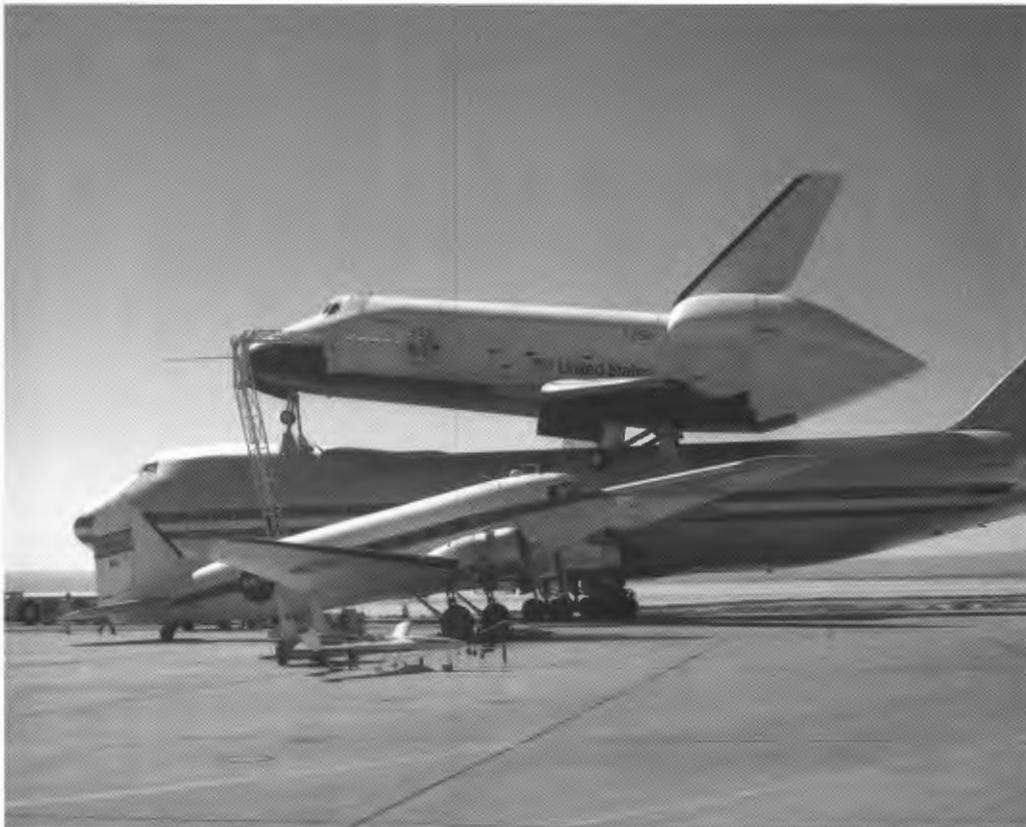
Three generations of vehicles in a row: in front, Dryden's Mini Sniffer, a small UAV designed for high altitude research, in the middle is Dryden's "new" C-47, and in back, the Shuttle Carrier Aircraft with *Enterprise* on top. The extra large cherry picker was to enable the shuttle crew to get into the orbiter. NASA EC77-8143
