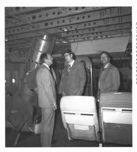
Standing on the main deck of the 747 Dryden center director Ike Gillam looks distractedly at the ceiling while two other VIPs chat. Behind them the emergency escape tube runs from the upper deck, through the floor, down to the side of the aircraft in the cargo hold. NASA E77-31893
