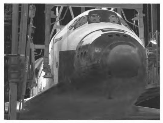
slingback, nearly ready for the final lift before lowering it onto the back of the Boeing 747 SCA. The landing gear has been stowed and the cockpit windows have been covered. NASA EC90-065-13
