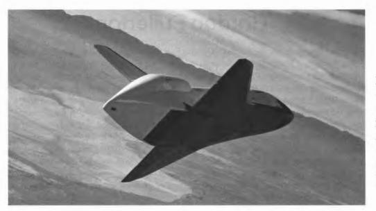
Enterprise in free-flight turning toward Rogers Dry Lake at Edwards Air Force Base. This is second of five free-flights, indicated by the presence of the tail cone on the orbiter. NASA ECN-8607
