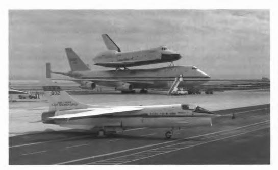
Dryden's F-8 Digiital Fly-By-Wire sits in front of the SCA and *Enterprise*. The F-8 DFBW was instrumental in solving the shuttle's latent PIO tendencies. NASA EC78-9354
