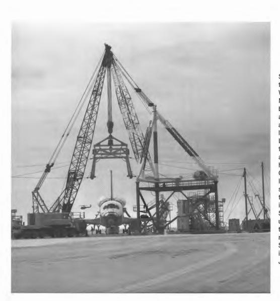
STS-3 diverted to Northrup Strip, White Sands Missile Range. because of rain at the primary and secondary landing sites. Lacking an MDD there, alternate arrangements had to be made. Cranes are lowering the slingback in order to lift Columbia in order that the SCA can be towed under it and the two mated for return to KSC. STS-3 post landing image courtesy of Joe D'Agostino
