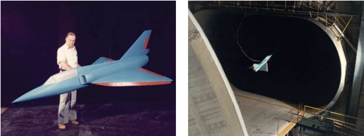
Free-flight model of the F-106B modified with a vortex flap (left) and in flight in the Langley Full-Scale Tunnel (right).
