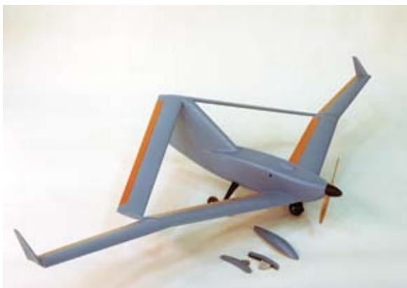
Advanced agricultural airplane model tested at Langley.
