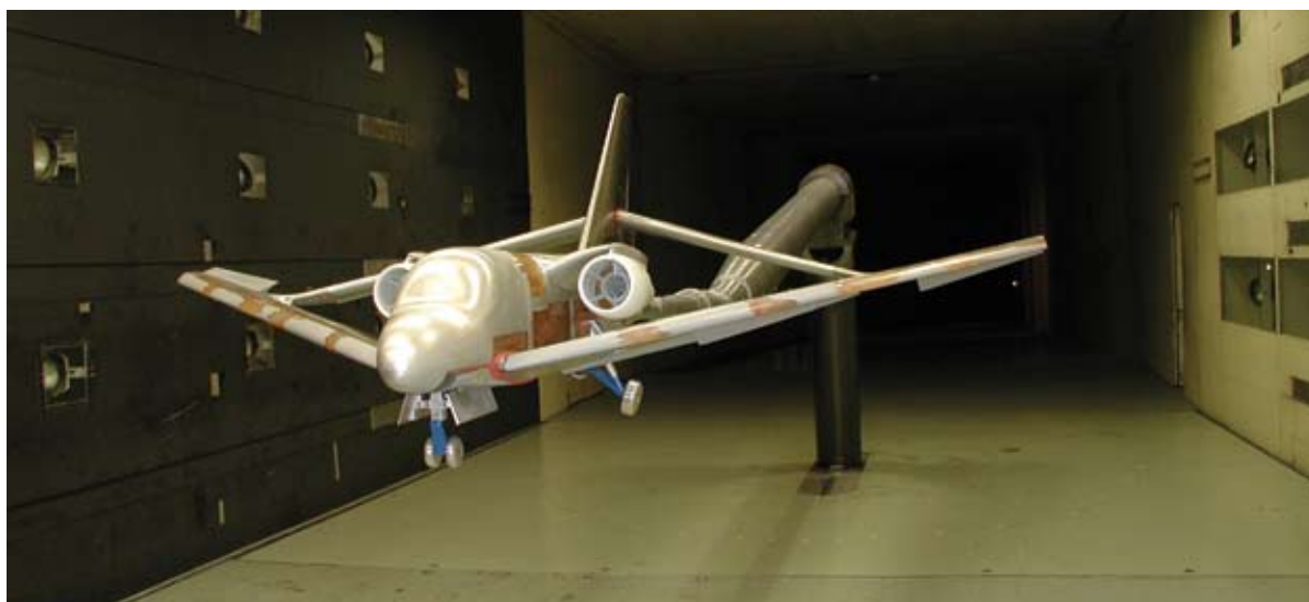
Model of the Joined-Wing Flight Demonstrator in the Langley 14- by 22-Foot Tunnel.
