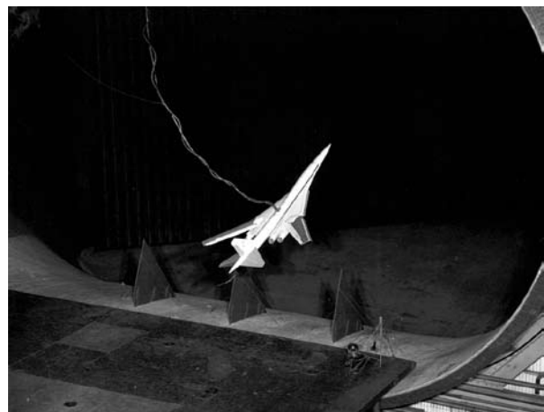
Time-lapse photography shows the variable sweep wing of early Boeing Model 733-290 Supersonic Transport design. Free-flight testing was conducted in the Langley Full-Scale Tunnel.
