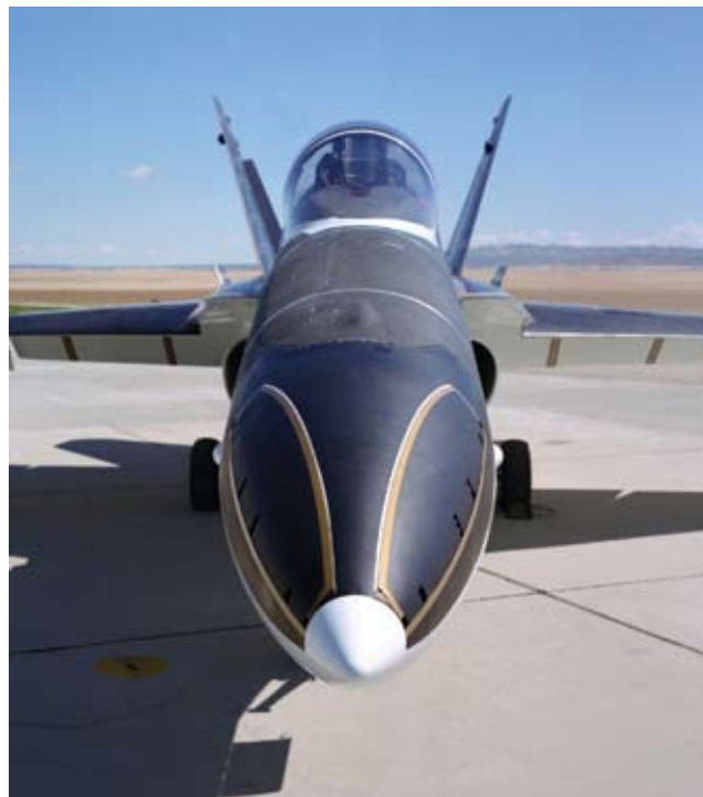
Close-up view of the forebody strakes on the F/A-18 High Angle-of-Attack Research Vehicle research airplane.
