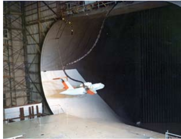
Technicians David R. Brooks and Benjamin J. Schlichenmayer prepare a free-flight model of a USB transport for tests in the Full-Scale Tunnel.
