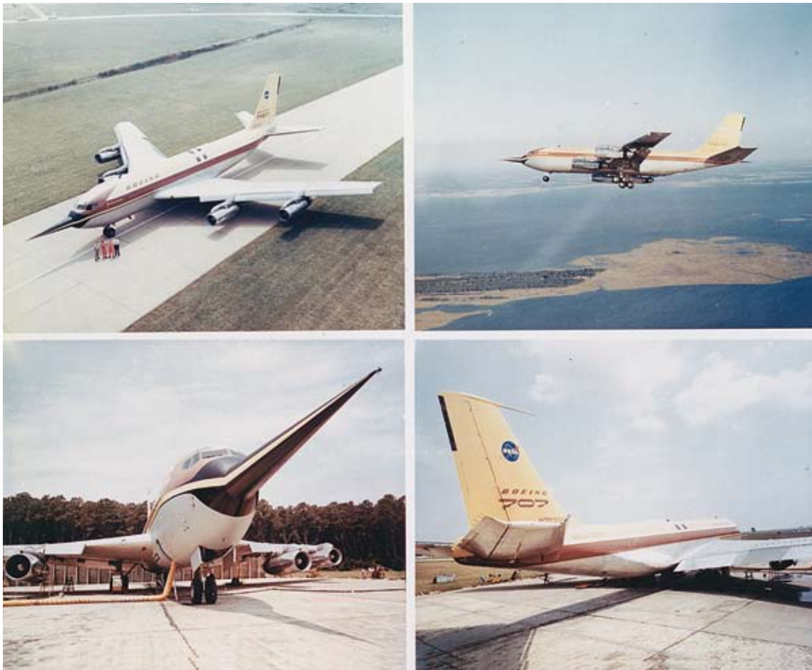
Boeing's 367-80 was used at Langley for in-flight simulator studies of handling qualities of supersonic transport configurations.
