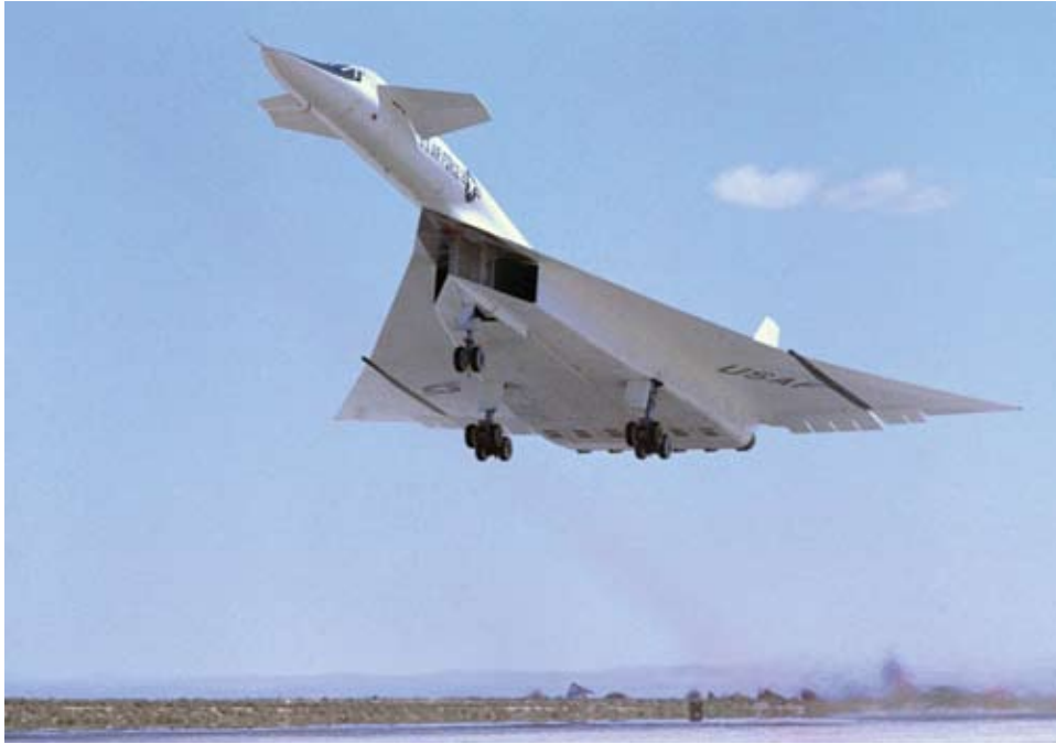
The XB-70 bomber, designed for supersonic cruise at Mach 3.0.
