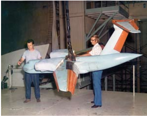
Technicians David R. Brooks and Benjamin J. Schlichenmayer prepare a free-flight model of a USB transport for tests in the Full-Scale Tunnel.
