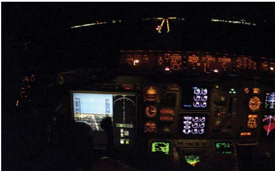
Night scene during practice flights for Dallas-Fort Worth showing SVS display and out-the-window runway lights.
