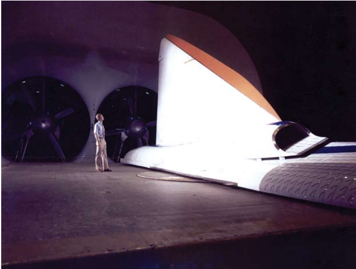
Neal Frink inspects full-scale semispan model of F-106 equipped with his vortex-flap design.
