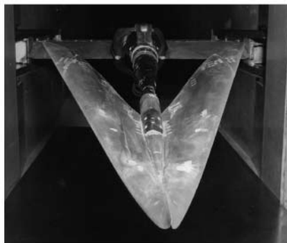
Highly swept arrow wings are nearly optimum shapes for supersonic flight.
