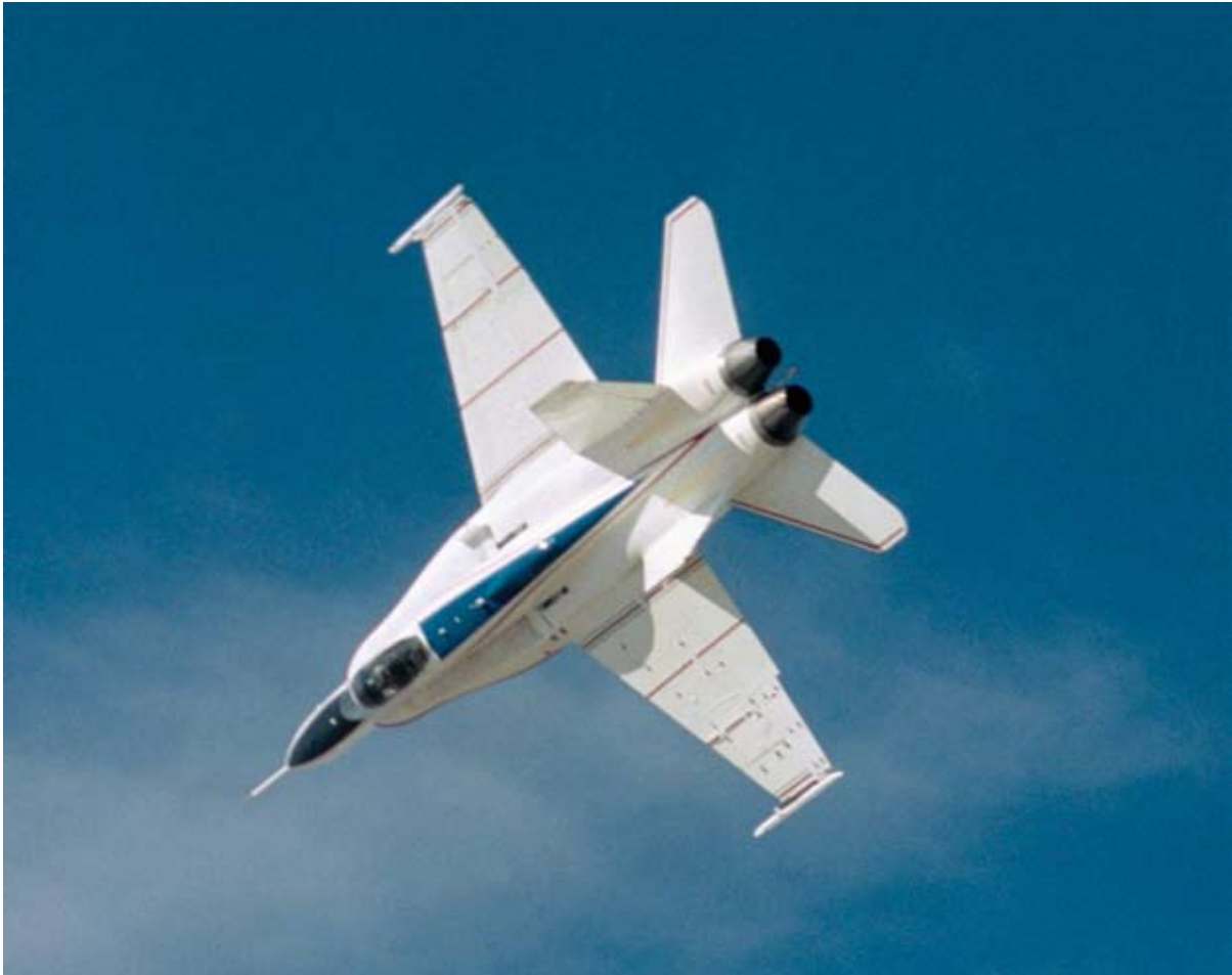
NASA's active aeroelastic wing F/A-18A research aircraft maneuvers during a test mission.
