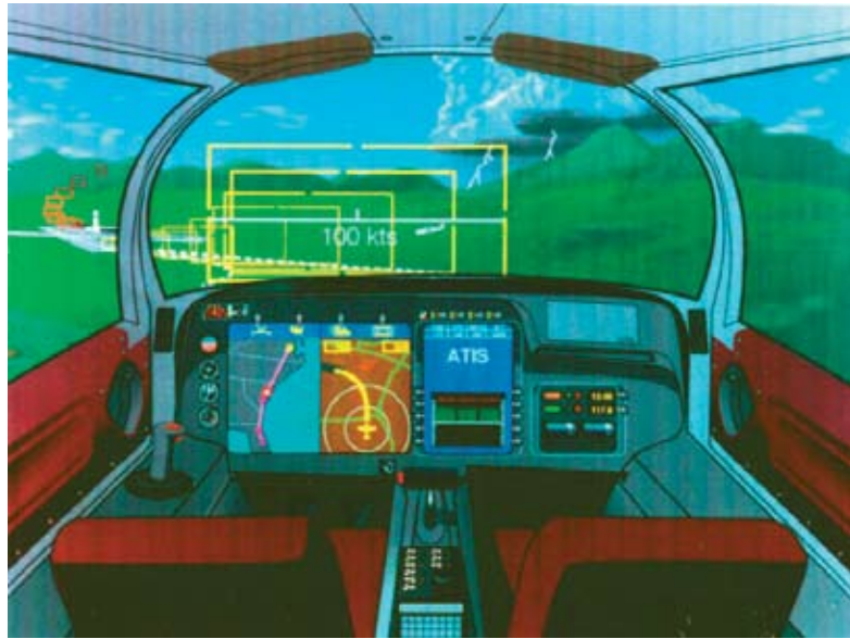
Highway-in-the-sky concept in NASA AGATE Program.
