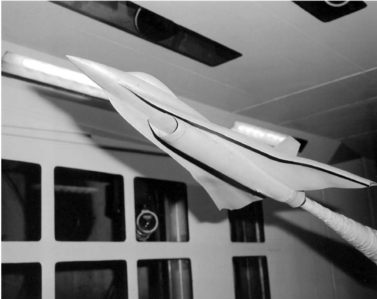
Camber study model used to develop optimum camber.
