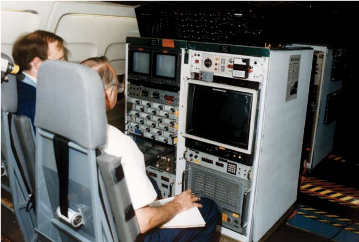
Langley researcher Dal Maddalon (right) and Boeing engineer David W. Lund (left) monitor wing transition data aboard the 757 during a typical research flight.
