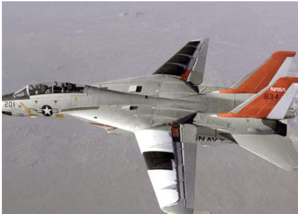
The F-14 Variable-Sweep Transition Flight Experiment airplane in flight with research gloves on both wing panels
