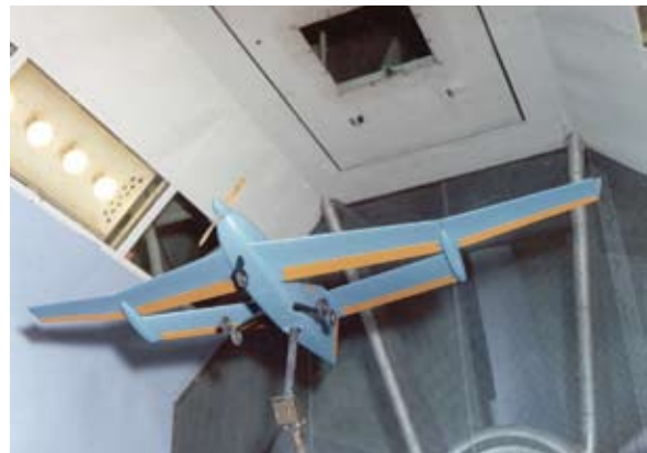
Advanced agricultural airplane model tested at Langley.
