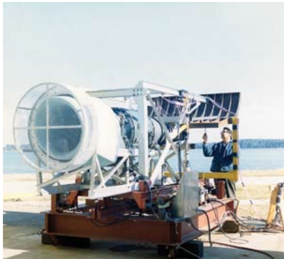
Engine test-stand investigation in preparation for tunnel tests of modified Aero Commander airplane. Photo on right shows turning of flow around upper surface blown flap.
