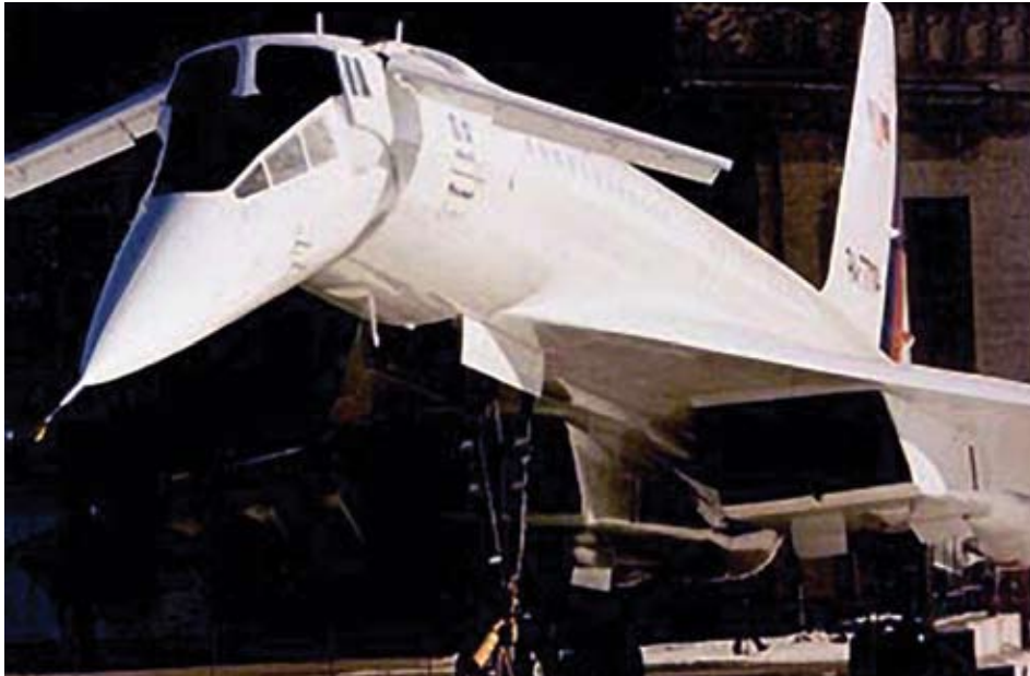
The Tu-144 supersonic transport used a variable-geometry drooped nose for improved visibility during low-speed operations.
