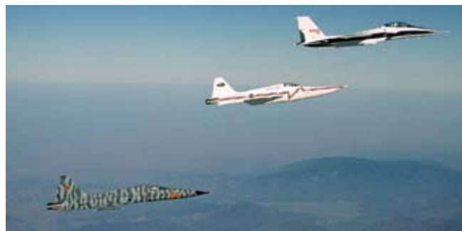
Aircraft used in the shaped-boom tests. From top: the NASA F-15B survey airplane, the F-5 shaped-boom demonstrator, and the baseline F-5E.
