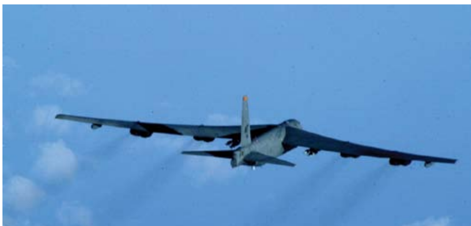
Photographs of B-52 airplane on the ground and in flight graphically show the structural flexibility of the wing.
