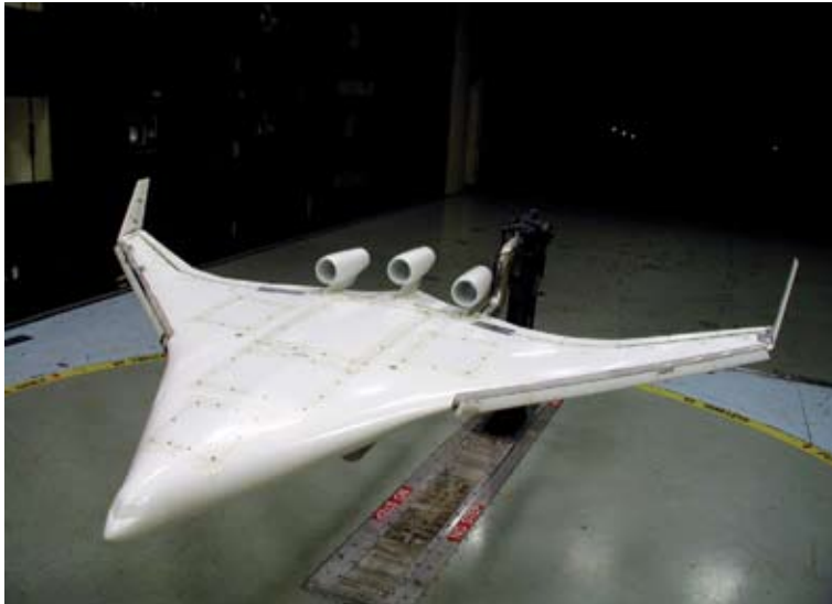
BWB-450 model used for initial tests in the Langley 14- by 22-Foot Tunnel.
