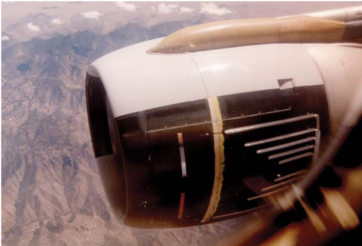
View of the instrumented CF6-50 engine during hybrid laminar flow control nacelle flight tests.
