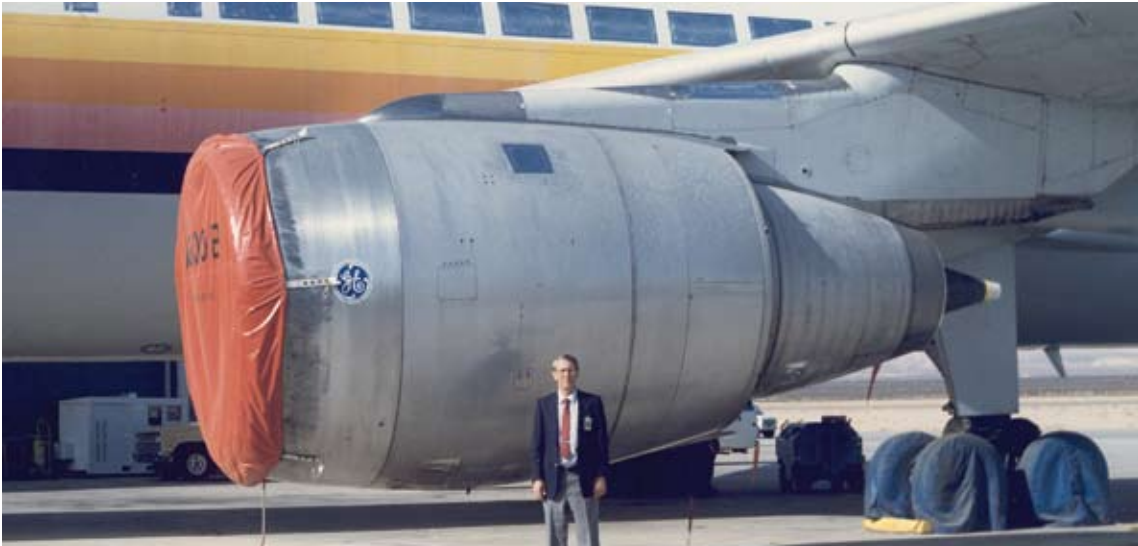
Relative size of Langley researcher Vernie Knight illustrates the massive size of the General Electric CF6-50 engine nacelle.
